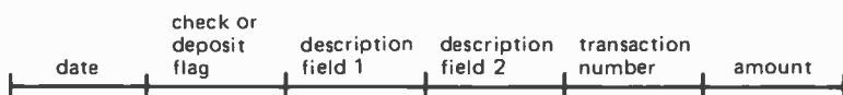
Figure 4: A sequential file with a record format such as this is the simplest physical data base for the checkbook program. The information that is needed has been decided by the logical data base. The order they are put on the file depends on exactly what you intend to do. Since in this case we will be sorting by date, the date of the transaction appears first on the file.
