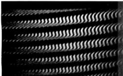
Photo 1: This is the display generated by the program written to output a series of vertical bars. The dark bands running across the monitor indicate that the horizontal frequency of the video interface and the horizontal frequency of the monitor are not identical.
