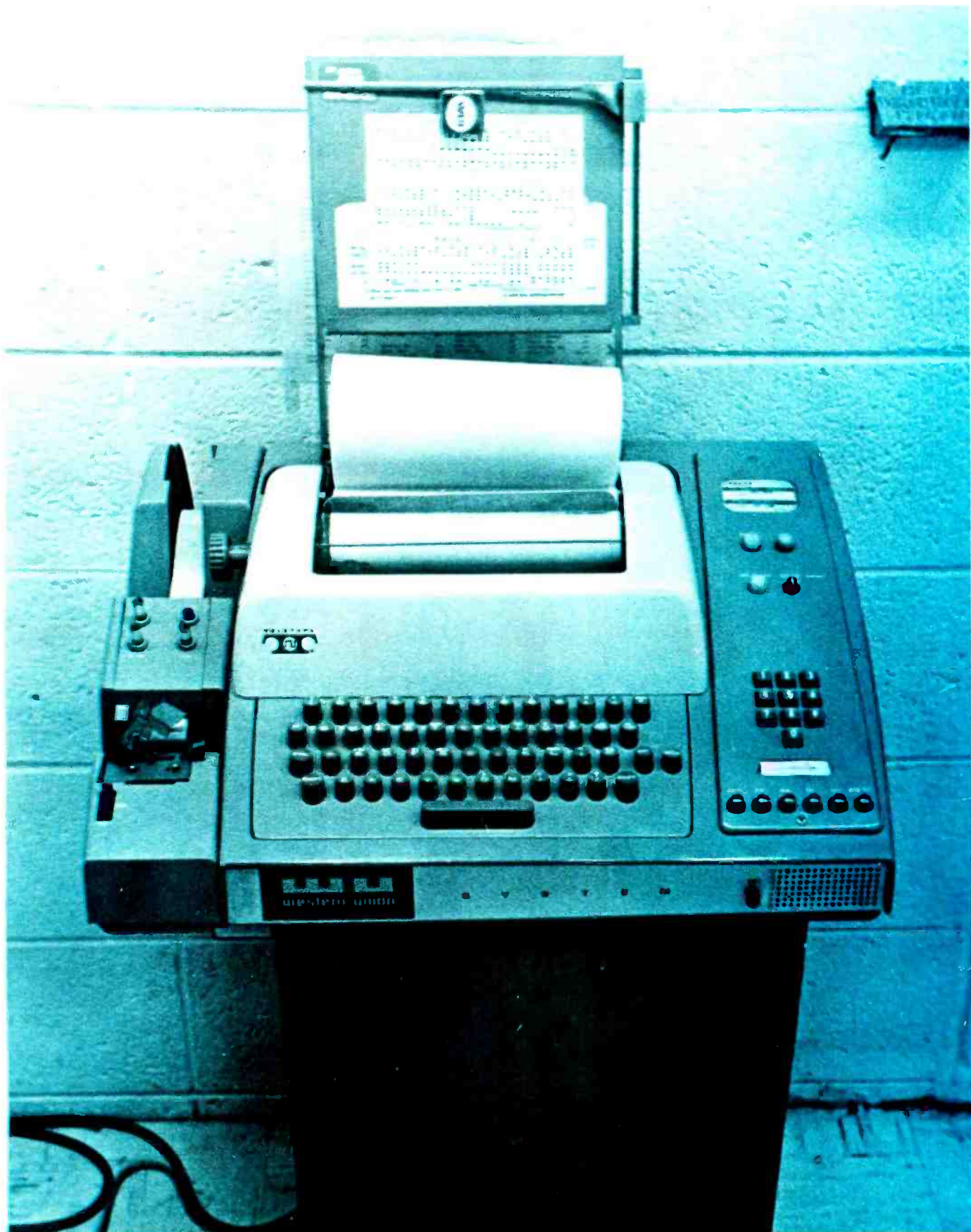
Photo 3: The "standard" Teletype so often seen in computer centers and personal computing contexts is the Model 33 ASR shown here with a modem option installed. This light duty machine is the war horse of the minicomputer world.
