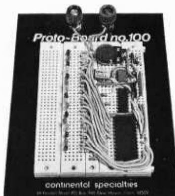
Proto-Board® 100. 760 solderless tie-points. Kit, $19.95*
