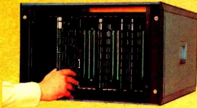
Full-width motherboard has slots for 21 cards.
