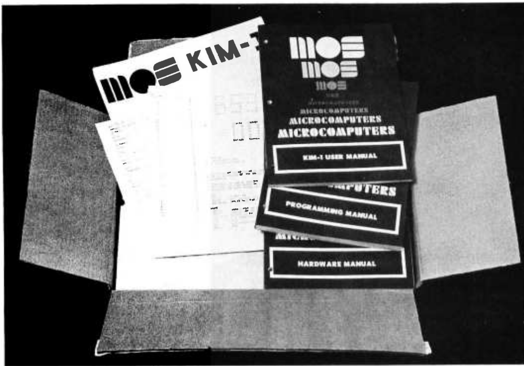
Photo 1: When you first open your KIM-1 box, you see a thick layer of documentation, including a large wall chart of the system's hardware details, an MCS650X Instruction Set Summary card, KIM-1 User Manual, Programming Manual and Hardware Manual. Also shown in this picture is the KIM monitor listing copy which must be requested separately and is a must if you are to take advantage of KIM's sub-routines in applications programs.
