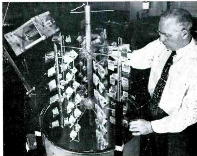
Like a cluster of glowing ice cubes, these seeds of synthetic crystals are about to be lowered into a growing tank at Bell Telephone Laboratories where engineers have developed a method of culturing them as a substitute for scarce but heretofore indispensable quartz.
