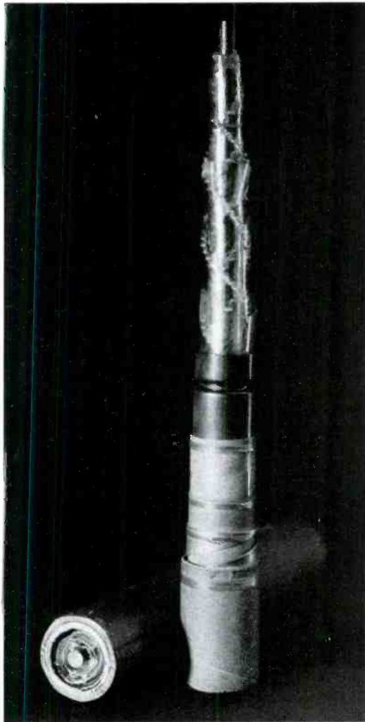
A section of German coaxial cable, showing elaborate use of styroflex insulation to suspend the central conductor in the pipe.
