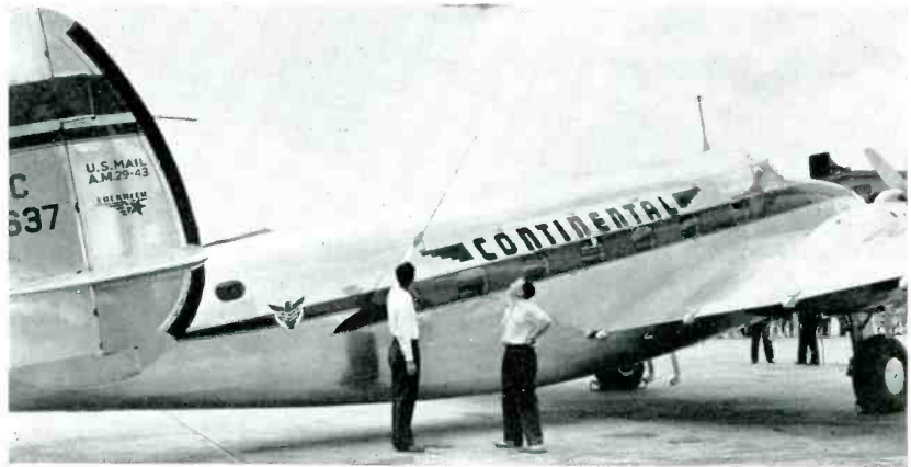
31 megacycle doublet antenna installation on Lockheed transport. Joe Rohrer making the inspection, Vern Andrews holding the transmission line to show how it bows in the slipstream when in flight
