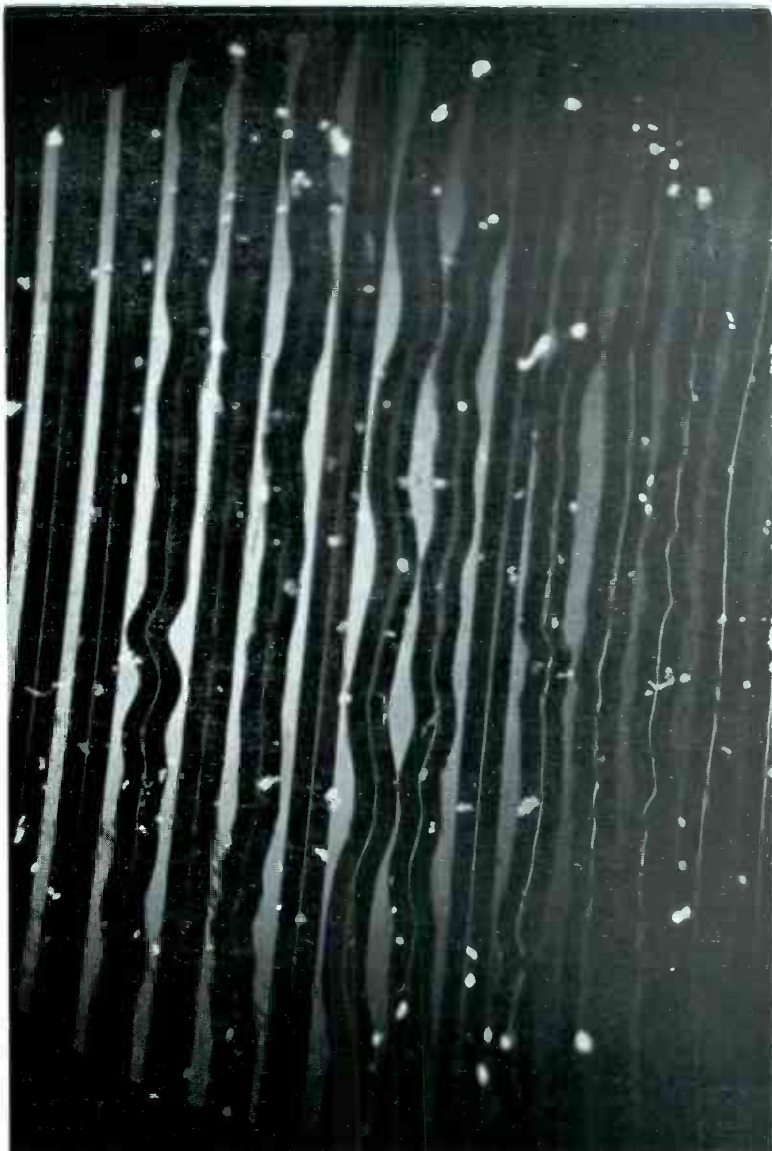
Lint particles removed from wiping cloth by sharp groove edges of freshly cut acetate.
