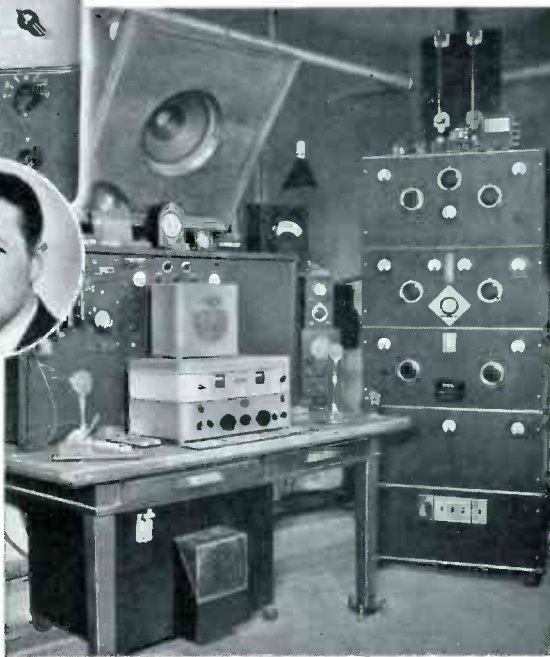
Outstanding transmission at 1 k.w. on each of 5 bands by "Tom" Consalvi's W3EOZ at Bryn Mawr, Pa., is matched by the perfect performance of his AR-77 receiver shown in the foreground before installation in the panel.
