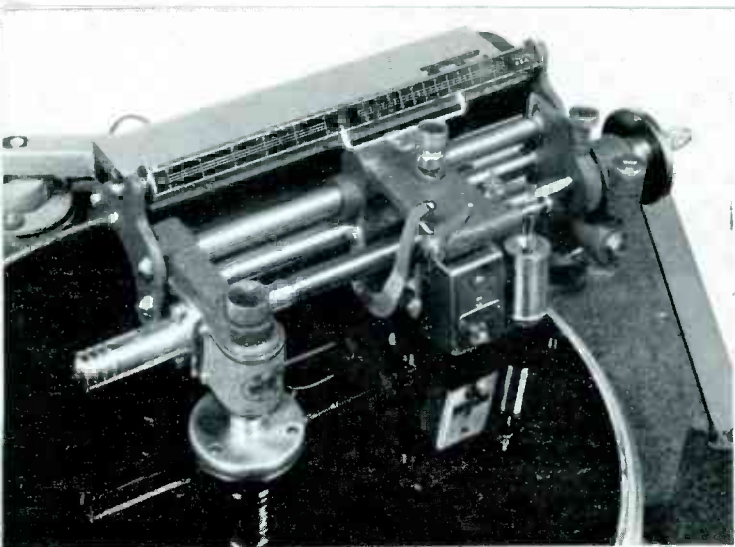
Fig. 8—Close-up of Feed Mechanism with New Type Equalizer attached
