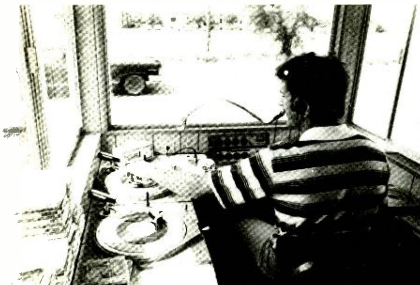
Inside the remote studio are two Russco turntables, two Collins cart machines, a receiver, Marti transmitter, Shure mixer board, and PA amplifier.
