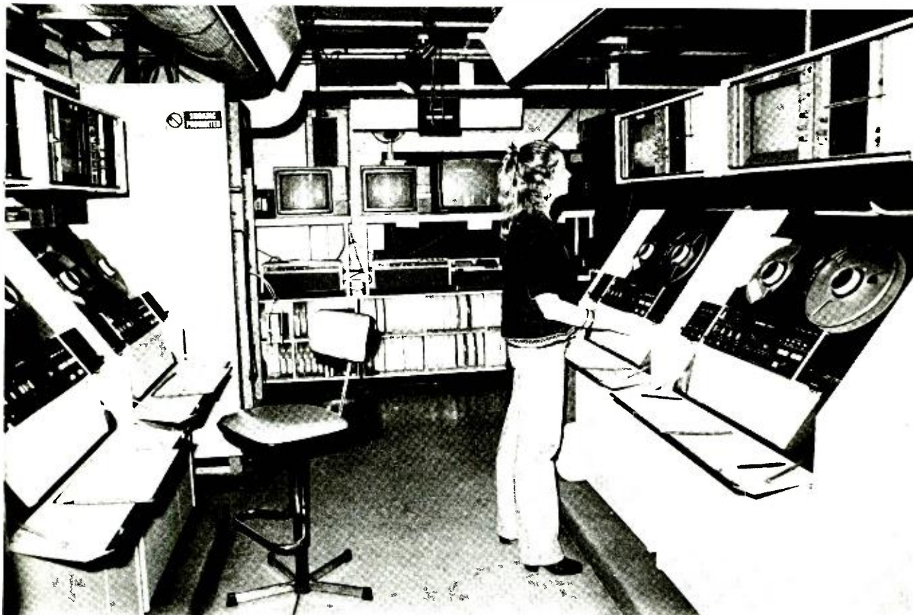
The new editing facility uses Ampex VPR2 one-inch helical Type C machines operating in PAL. U-matics in the background are for news editing of material shot in that format.
