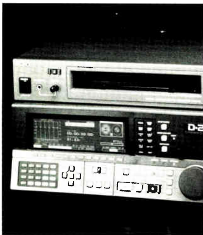
Viacom has three of the above DVR-10 Composite Digital Recorders in its all-D-2 environment.
