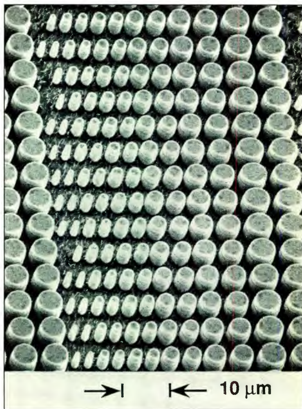
This hair-thin section of the Bellcore/Bell Labs chip contains more than one million working lasers per square centimeter.
