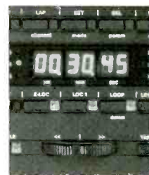
Timer-autolocator control panel
