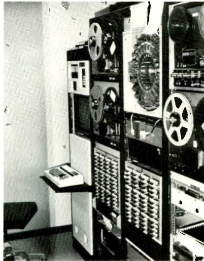
The satellite automation system at WWJR in Sheboygan, WI, showing Instacarts in lower foreground and ICM Basic III controller at rear.
