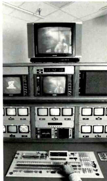
Utah Scientific's SAS-1 station automation system works in conjunction with the MC-500 series of master control switchers.
