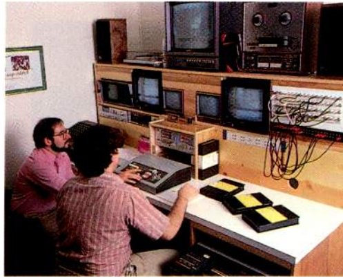
Locus Communications' 3/4-inch JVC/Convergence suite provides filmmakers with cuts-only editing. According to executive director Gerry Pallor, "They actually like straight cuts."
