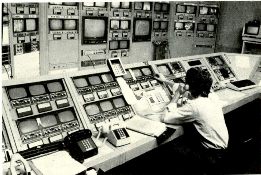
The Vernon Valley network monitoring center checks all video programming on RCA spacecraft and can determine if signals are being transmitted on spec.
