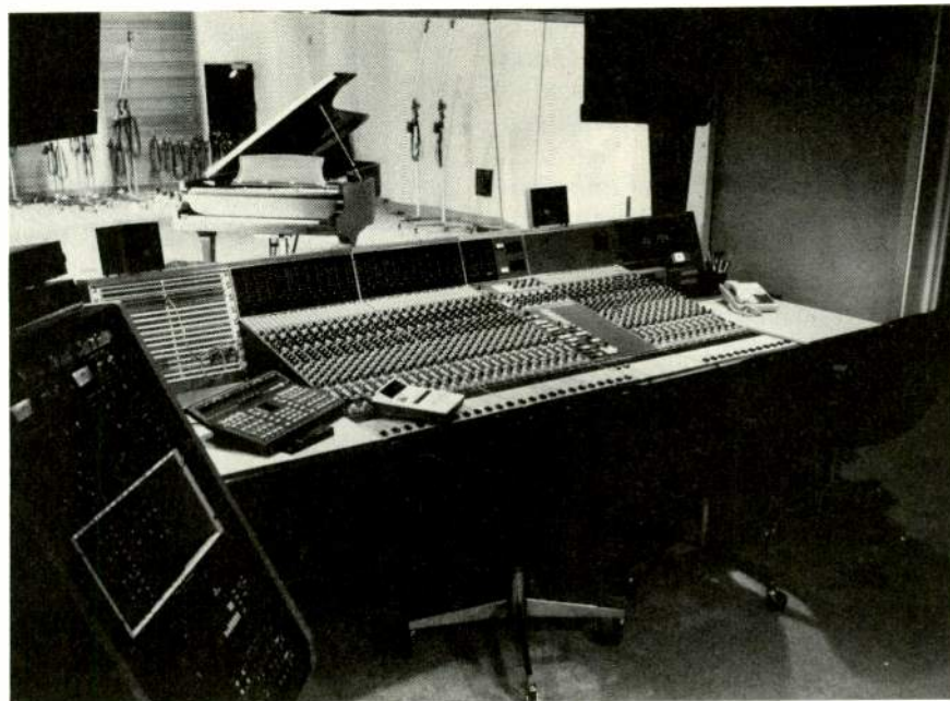
A Neve console is the newest addition to MPR's multitrack recording setup.
