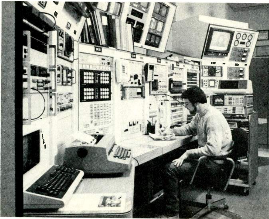
A portion of the communications console at RCA's Vernon Valley, NJ, earth station, where personnel monitor the uplink and downlink of DATS and SCPC radio transmissions.
