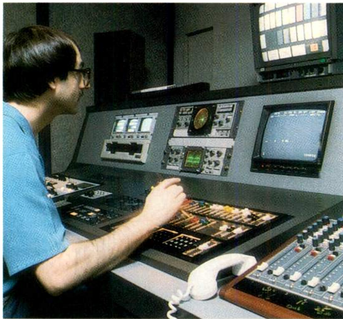
The industry most likely to reap immediate benefits from the new D-1 digital technology is teleproduction. At New York's Windsor Total Video, a technician operates a digital color correction machine.
