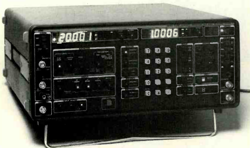
Automatic distortion and noise measuring system for Amber Electro Design's 5500 Series.
