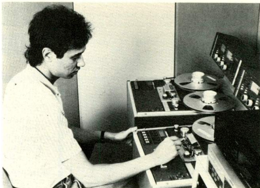
A Studioline Cable Stereo technician prepares one of the facility's 48 Studer A810 audio recorders for recording of program master tapes.
