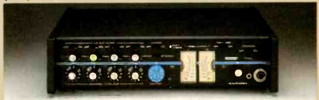
The new FP42 Stereo Production Mixer — the stereo counterpart to our M267. Four channels with independent center detented pan pots and cuing. Headphone amplifier. Adjustable limiters.
