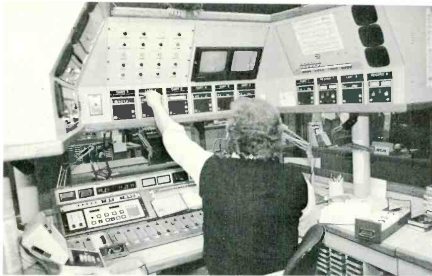
DJ Randy Jay in the KIMN/KYGO control room, which utilizes Howe Audio 24-channel consoles in addition to the three-sided overhead cockpit turret cabinetry, which contains eight ITC Delta single-play decks.
