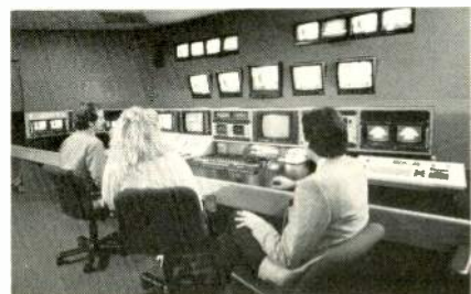
The Post Group's Edit Bay 6, with GVG 300 switcher and CMX 340C editor, can simultaneously summon up to four channels of ADO, Mirage, and NEC DVE Mark II.
