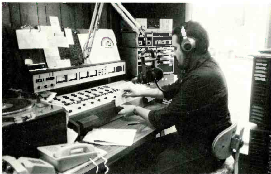
A new Harris Medalist Board, Technics SP-10 MK II turntables, and ITC cart machines geared WWNR for AM stereo production.
