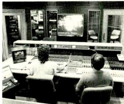
Sweetening Room A at the Post Group gives operators eye contact with the machine room (left) and the announce booth (right). The suite has a Neve 8128 automated console, CMX edit control, and Otari recorders.
