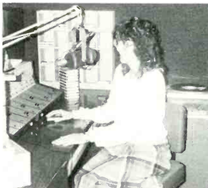
In the station's main control room, the Centurian II board was upgraded for stereo. The ITC cart decks in back were already geared for stereo playback.
