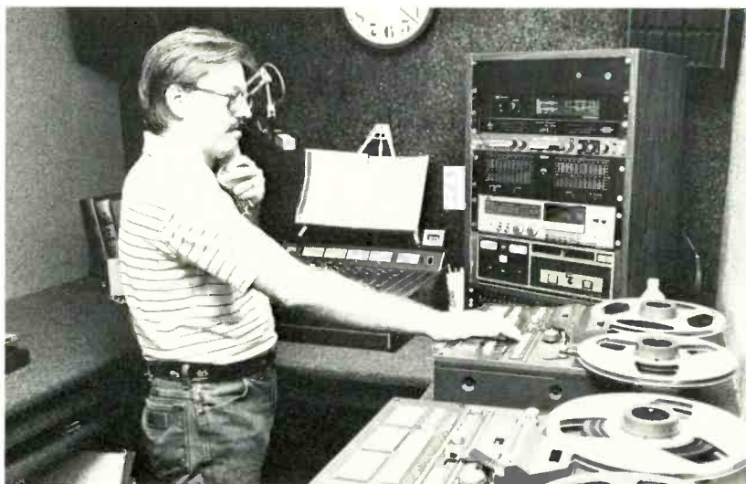
Special effects production room includes EQ, digital delay, flanging, compression, and stereo enhancement. Recorders are four-channel Teacs.
