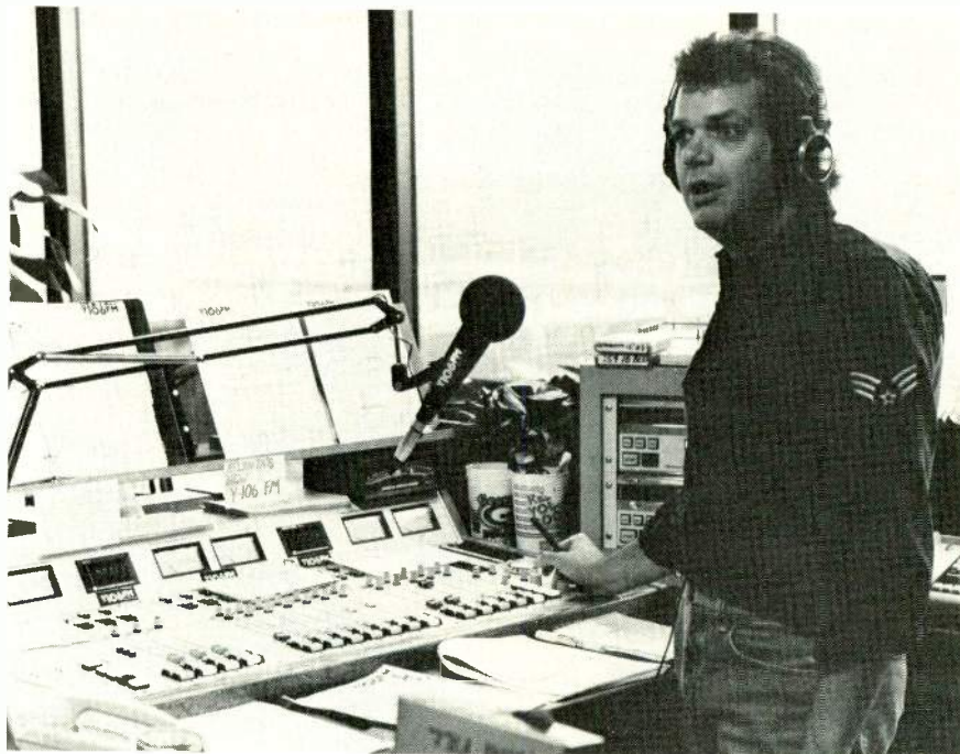
DJ Johnny "Stonewall" Jackson in the air studio, which is built around a Pacific BMX-III console, six Tomcat cart players, and two Technics turntables.
