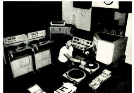
The production room centers around a Pacific Recorders BMX II 14 fader board. Turrets on either side of the board contain an Orban 424A compressor/limiter, 111B stereo spring reverb, and an Eventide H949 Harmonizer.
