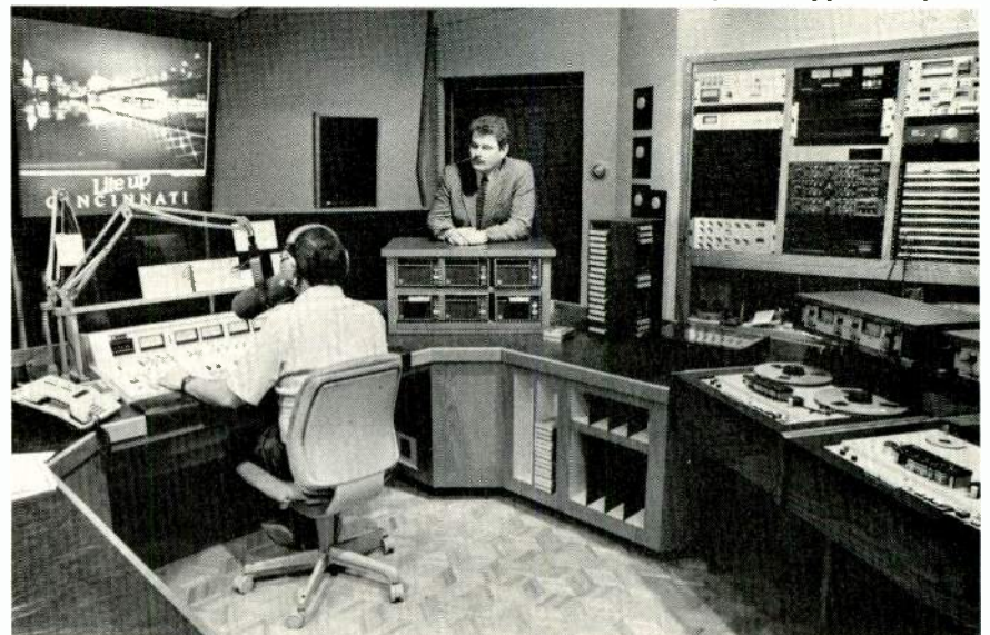
WLLT's air studio features oak cabinetry custom-built by the Audio Broadcast Group. To the right is a housing with special slide-out shelves for six ITC-99B cart machines; two Sony CDP-650 CD players; and two Sony two-track machines.
