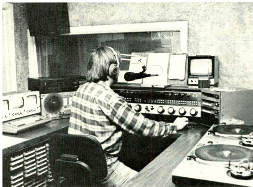
KTAM control room features video monitor (left) that displays the front door, UPI messages, and local zone weather forecasts. Technics turntables are used for special programs.
