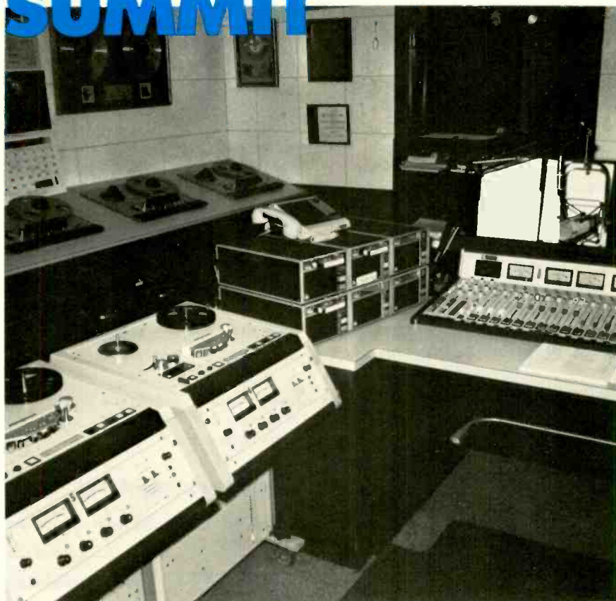
WTQR's upgraded control room features a custom Auditorics 200 Series on-air board, along with Otari ATRs and ITC 99 Series cart machines.
