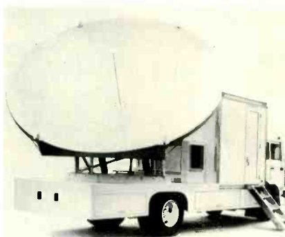
Dalsat transportable Ku-band uplink for Florida News Network. The 4.5-meter dish folds for storage.
