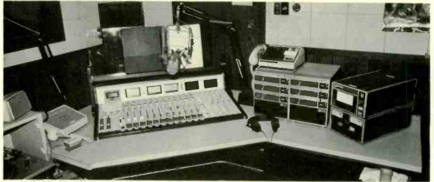
WSJS and WTQR share the news studio, which is built around an Audiotronics 200 Series console similar to but smaller than the ones in the control rooms. Turntable at far left is a Technics SP-10.
