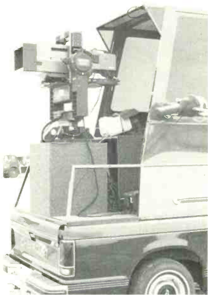
Winged Vision's gyro-stabilized camera mount is affixed to the back of vehicles for marathon coverage.
