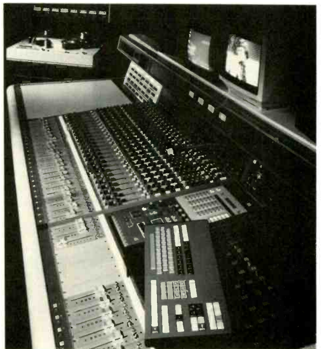
Neve Necam 96 console automation system.
