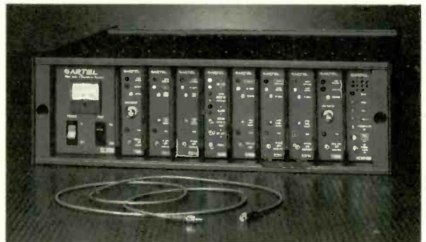
Artel laser-based fiberoptic system.
