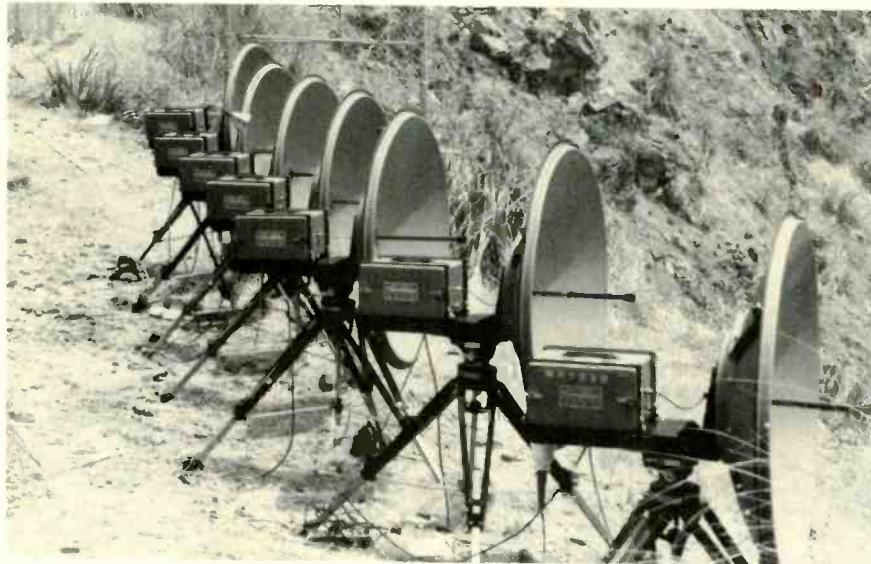
Aligned with microwave transmitters atop San Francisco's Moscone Convention Center 13 miles away, these antennas relayed live TV coverage of the Democratic National Convention to TV stations across the country via three Bonneville Communications transportable satellite uplinks.
