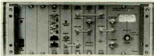
LKFM01 - TRANSMITTER, 1.7 - 2.5 GHz, 1 VIDEO - 2 AUDIO
