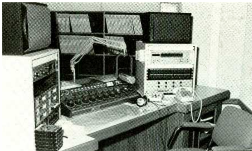
Air control utilizes an MEI event controller, visible at top in the right-hand table rack. The Broadcast Electronics console allows manual override of the mini-automation system.
