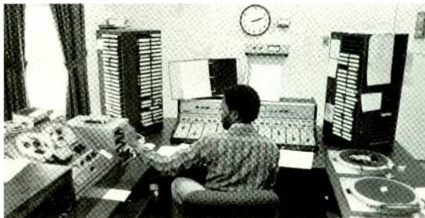
In the control room, program director Marvin Henry inserts a cart into the ITC three-deck cart machine. New equipment purchased for this room included the 10-channel Harris Medalist console at center.
