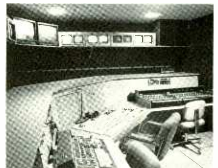
The studio control room includes a Grass Valley switcher and a 3M D-8800 two-channel character generator.
