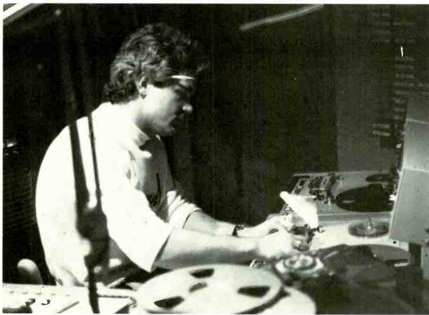
WLOL promotion director Tom Gowan at work in production. In addition to the ADM console and twin Otari MTR-10 ATRs, the room is equipped with a four-track Otari MX-5050BQ, used for special projects.
