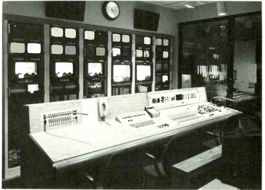
Studio A's control room can seat nine people. It features an ADM 24 console, a Grass Valley 300-3A switcher, and a Quantel DPE-5000.
