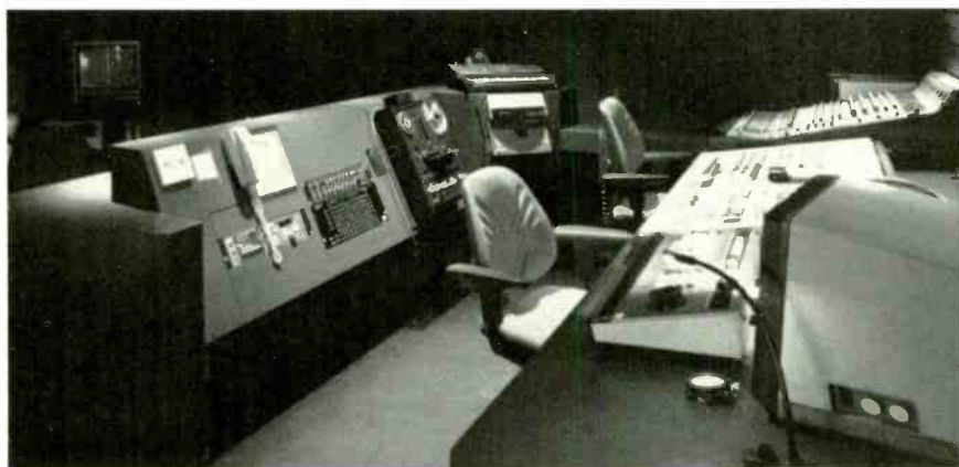
Edit Room One features a CDL-480-8 switcher, ADO and NEC digital effects, and a custom-modified Yamaha mixing console.
