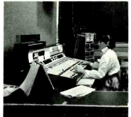
Station manager Carol Ross keeps things rolling from the Broadcast Audio System 14 console in KPEL's control room. Sitting on top is the Heath-Zenith weather computer.
