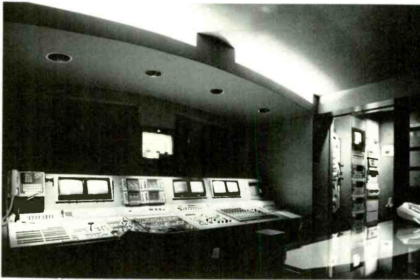
Color Correction Room 1 features, from left: a CDL-680 switcher, Dubner color correction, controls for a Rank Cintel MK-IIIC telecine, and a Neve audio board. Pictured in the room next door is a Rank Cintel Ferrit stereo dubber, and a bank of cassette decks.
