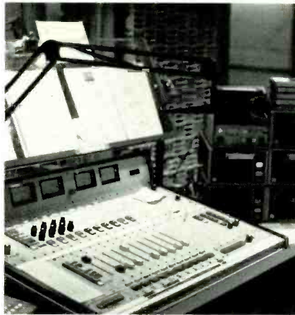
Station's control room features new ADM console and ITC cart decks. Window gives visual contact with lobby, keeping the station's product "up front."
