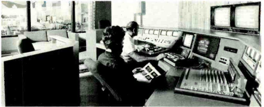
Edit 3, the largest and most sophisticated of Video West's three post rooms, features CMX 340X computer editor, Grass Valley 300 switcher, and ADO.
