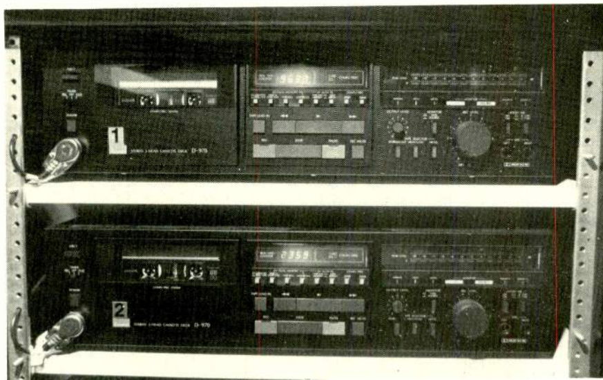
Sansui's D-970 consumer deck, one of nine on-line in KCMJ's FM Systemation setup.
