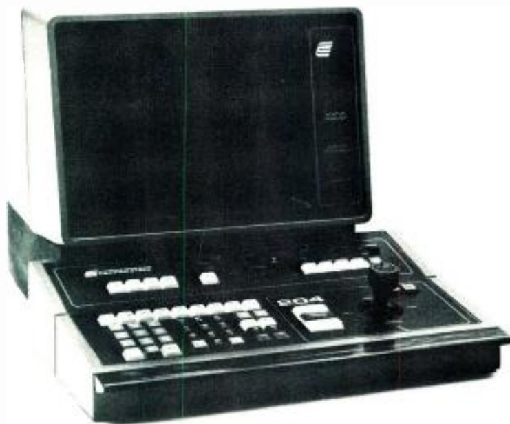
ESC-204 editor, with characteristic Convergence joystick.
