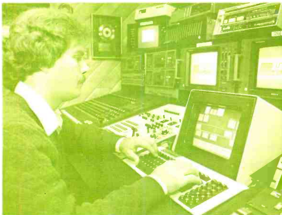
Bob Head at Henderson-Crowe's LightFinger Plus. Operator can interface system through screen, keyboard, or directly through tributaries (to right of program monitor).
