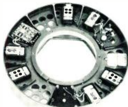
The upper drum with head/electronics assembly. Heads are field replaceable.
