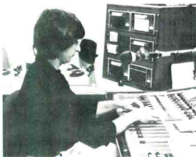
KWK-FM control room, pictured above, features a remote-controlled McCurdy SS8600 console, ITC Series 99 cart machines, and Panasonic Technics SP 10 MKII turntables
