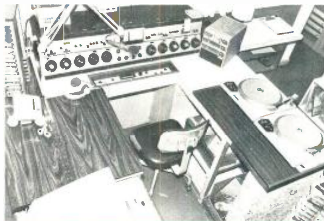
The main console area provides more space for the DJ and for interviews. Revox reel-to-reel is under the hinged lid at left. The five by five-foot carpeted backdrop at rear of console softens control room acoustics noticeably.
