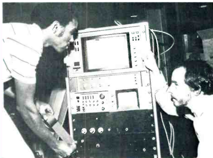
A field production crew (bottom, right) prepares to remove the "coffin" from the production van. The color monitor, CCU, scopes, mic mixer, and power supply are housed in an Anvil case for portability
