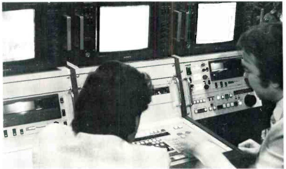
Demonstration of Sony's new editing system showing complete interfacability of BVU-800 deck (right) with new Betacam 1/2-inch player (left)
