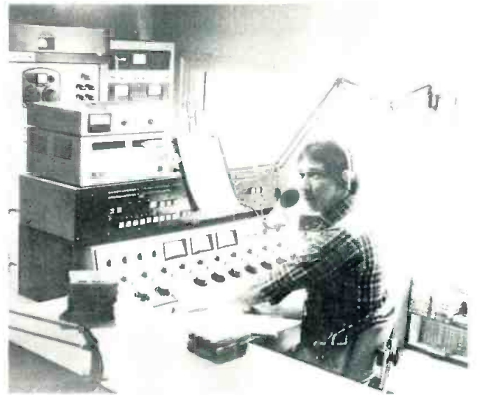
The control head above the 10-channel, modular Collins mixer was designed and constructed to allow the operator to monitor operations of either KOJM-AM or KPQX-FM and to instantly access either With a small staff and a diverse audience, the physical layout of KOJM/KPQX is set up for maximum observation with minimal separation of engineering components
