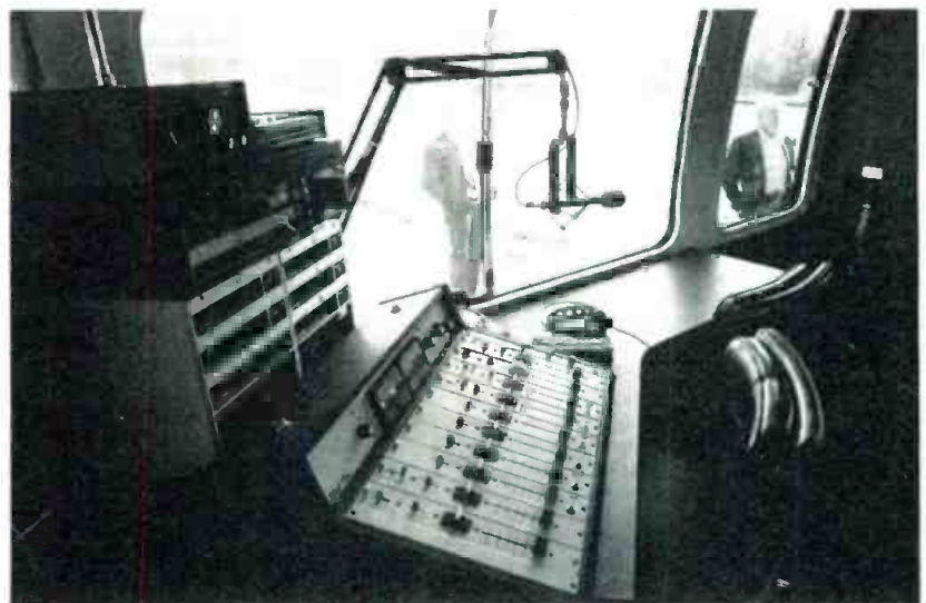
Interior of control position in WHDH mobile studio shows control console, record racks, and receiver for link to main studio. Turntables and cart machines are on operator's left; comfortable seat to his right is for interviewees
