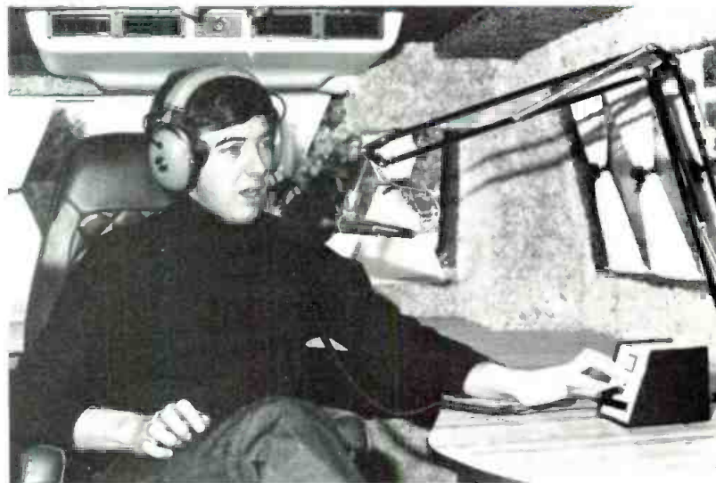
Rear of WROK van has attractively finished walls with sound absorbing material to create good studio acoustics. Space is allowed for comfortable seating of person to be interviewed, or to deliver "live" commercial
