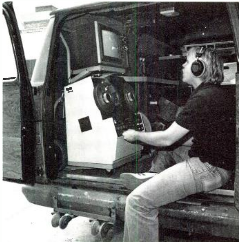
KSL Video Production's mobile van with Ampex one-inch recorder. VTR is mounted on a dolly, together with color monitor, and can be hoisted out of the van with a permanently installed winch, then wheeled to the location. VTR is powered from batteries or external ac
