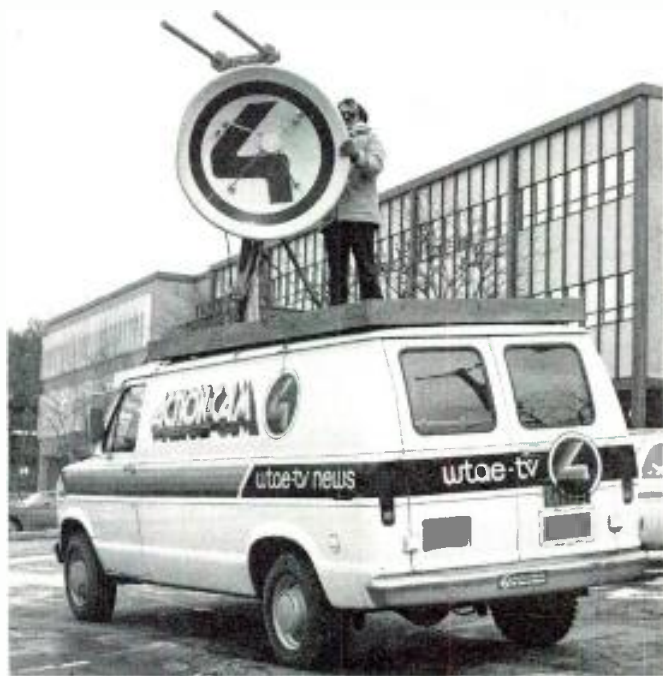
WTAE's first ENG/EFP mobile unit was fabricated at the station. This typical van was one of the first to be adapted to the new role of mobile repeater station
