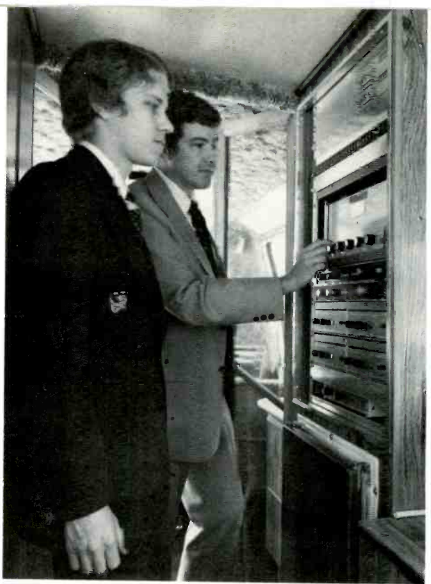
Technical assistant Jeff Weissert (left) and chief engineer Tom Monahan shown at the equipment rack adjusting the 450 MHz Marti RPU
