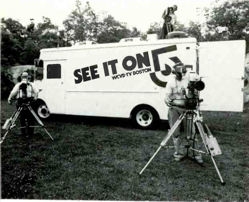
The Hippo carries three cameras: two Ikegami HL-51's, shown tripod-mounted, and an RCA TK-76, shown mounted on the roof
