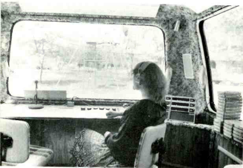
Studio area showing talent operating position to right and guest position to the left. Operating controls for the talent are directly in front, with the ITC cart machines to the right
