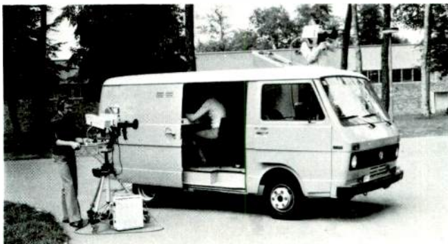
Compact OB van with 2 cameras KCK/R and 2 VTR BCN 40/50
