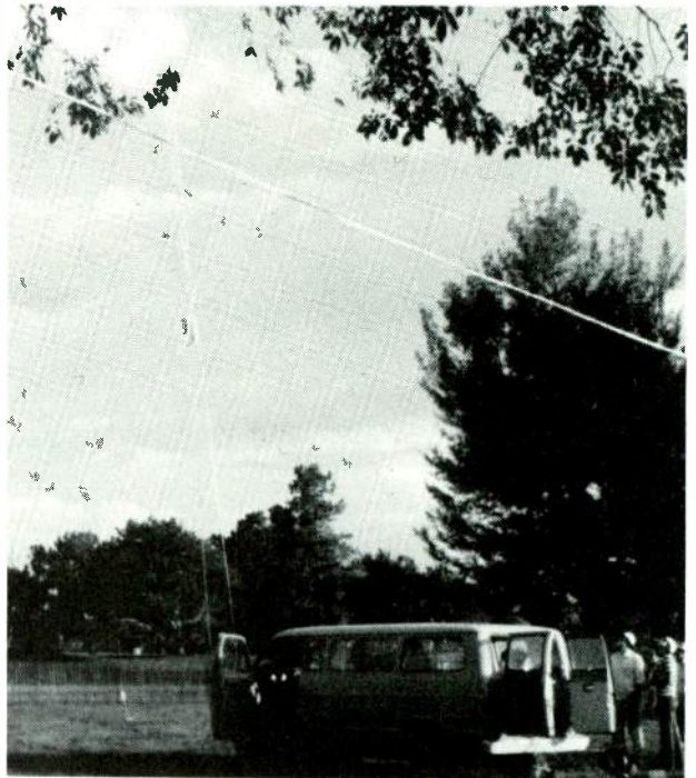
The van is the balloon's "anchor" and also houses the rear end of the microwave receivers. Power and signals are carried to the balloon via cables run with the tether
