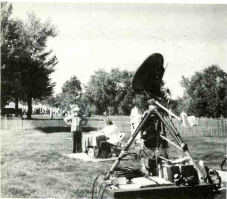
The platform which carries the antennas, m/w receiver front ends, and 950 MHz transmitters is made of a special lightweight material. ABC's Korn believes it could accommodate up to ten camera feeds
