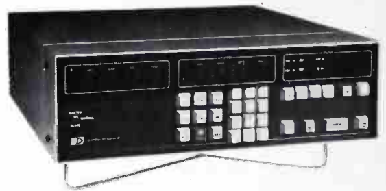
Fig. 10 EDS-200 editor/synchronizer incorporating microcomputer.
