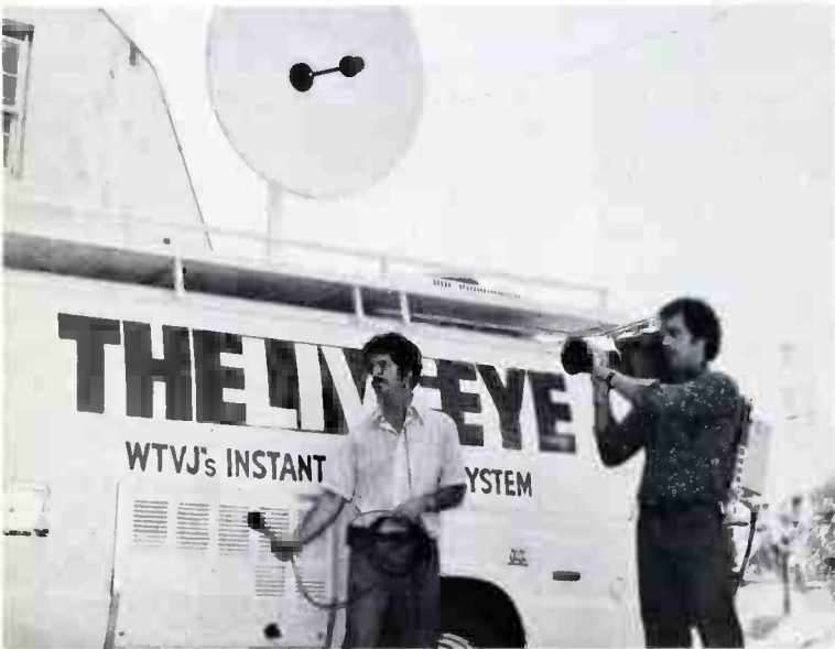
The WTVJ remote van prowls the Miami coastline with its Ikegami cameras, Sony 3800 VTR's and Microwave Associates dish. Signals can be transmitted to the main studios or to their Ft. Lauderdale transmitting facility.
