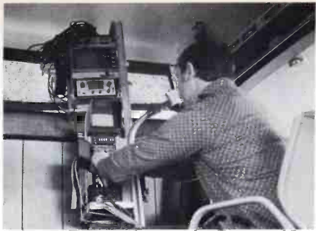
The video cart remains in the van for some taping jobs. Equipment from top to bottom: Shure mixer, five-inch Sony receiver modified as monitor (to verify color), portable Tektronix oscilloscope and waveform monitor; SK-70 backpack with standard viewfinder; Sony 2800 portable recorder; ac power pack for recorder, not shown.
