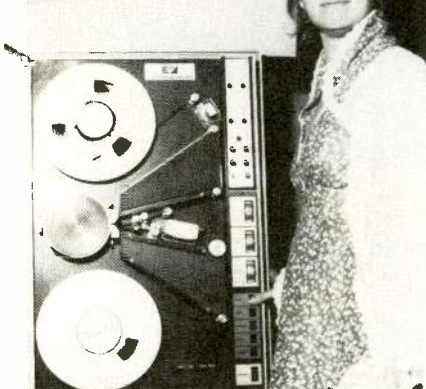
Video Memory's vacuum-buffered helical deck. 265
