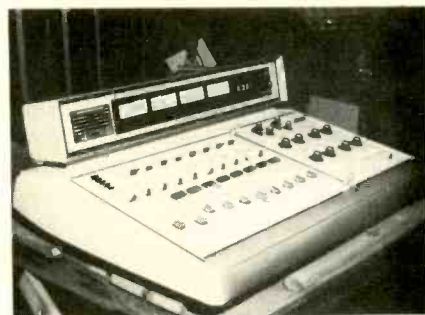
Cetec's 10-channel console has slide faders. 232
