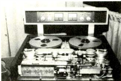
Studer's A-80 open-reel tape recorder was opened for inspection.
