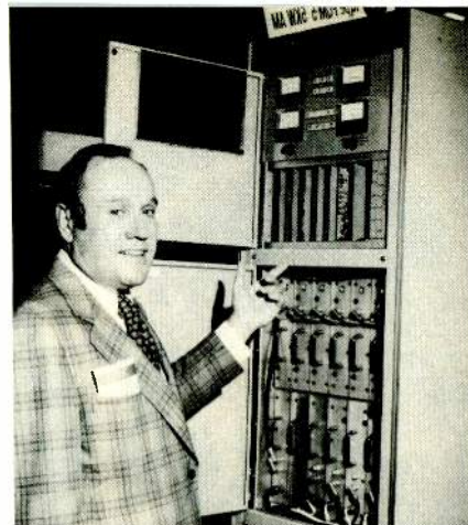
Westinghouse all-solid-state 5 kW AM transmitter. 210
