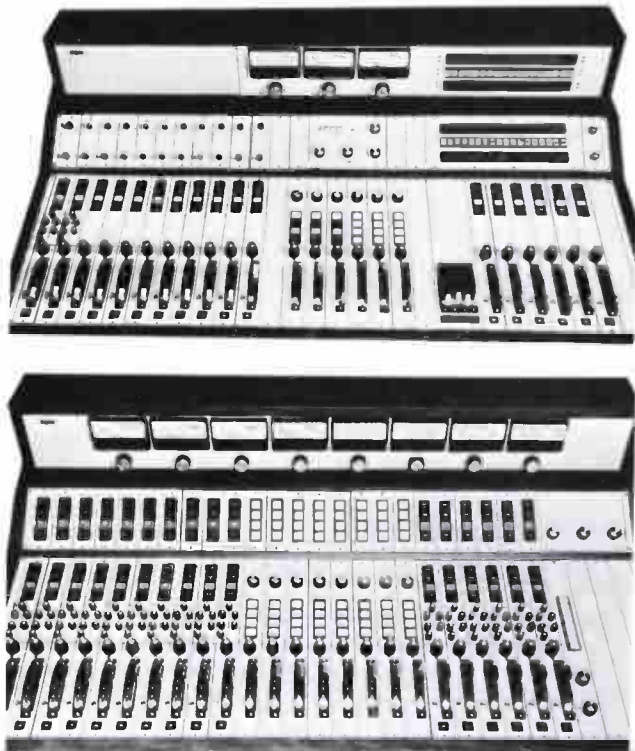
(Top) Custom audio console for WBEN-TV, Buffalo, has 11 inputs consisting of 11 pre-amps and one 6 X 18 high level input select panel. All channels have mixer modules (two with equalizers). Six have submaster modules. There is a custom built four-input telecine mixer. Monitor pushbuttons can look at three program channels. Unit has built in test oscillator.
