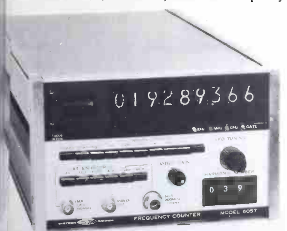
Coverage counter of extremely high accuracy is exemplified by Systron-Donner 6057, 20 Hz to 18 GHz, for monitoring of any frequency used in broadcasting or microwave relay work, with 9-digit readout.
