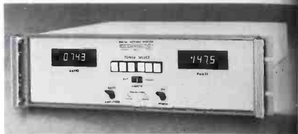
Other directional-array monitoring system so far approved by FCC is Delta Electronics, DAM-1 above. Operation is digital, as described in story.
