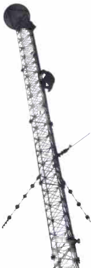
Dissipation array forms umbrella on top of tower at CKLW. Each of five towers in the directional antenna system is protected.
