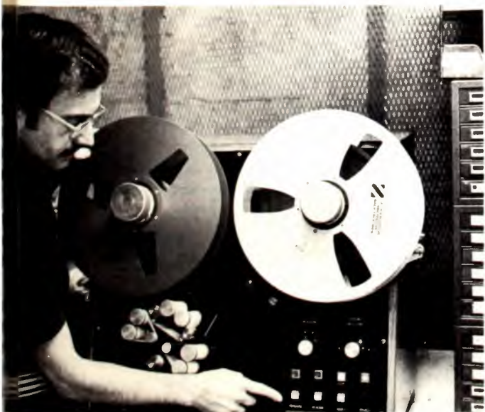
Magnetek tape cleaner is used on all videotape coming into WPIX from the outside. Shown here is Eric M. Heineman, technical director at WPIX.
