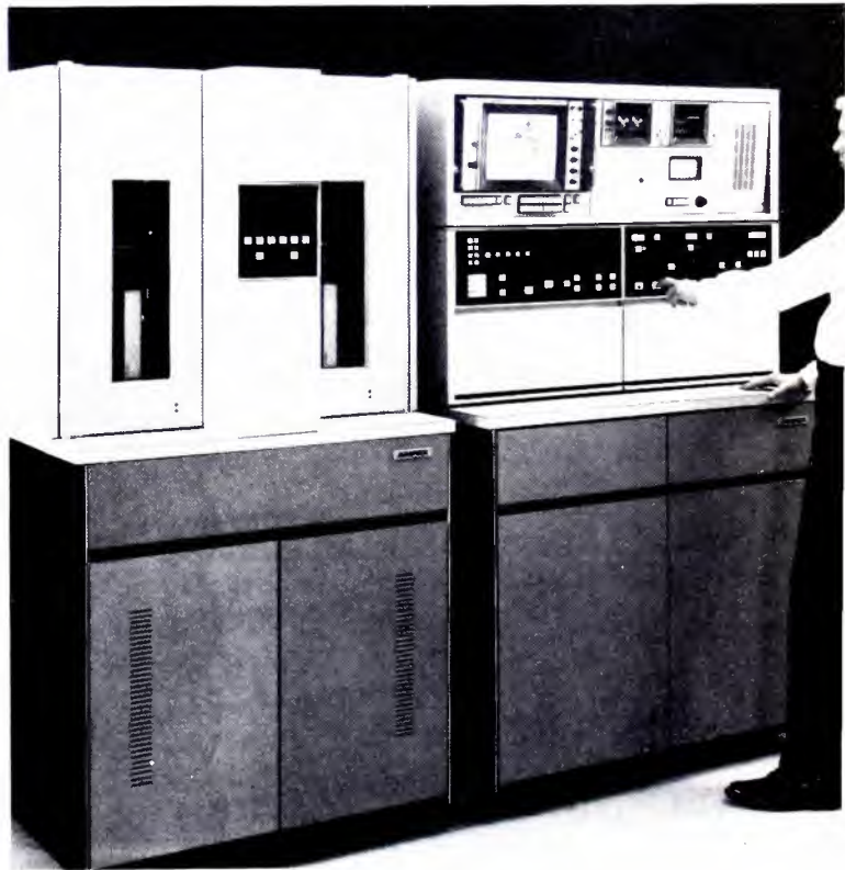
Ampex's simulated "on-air" newscast during the last NAB Convention demonstrated how news, sports, commercials, and promos can be incorporated into a fast-moving news show using the ACR-25 and AVR-1. The ACR-25 provides random access to up to 24 programs ranging in length from ten seconds to six minutes.
