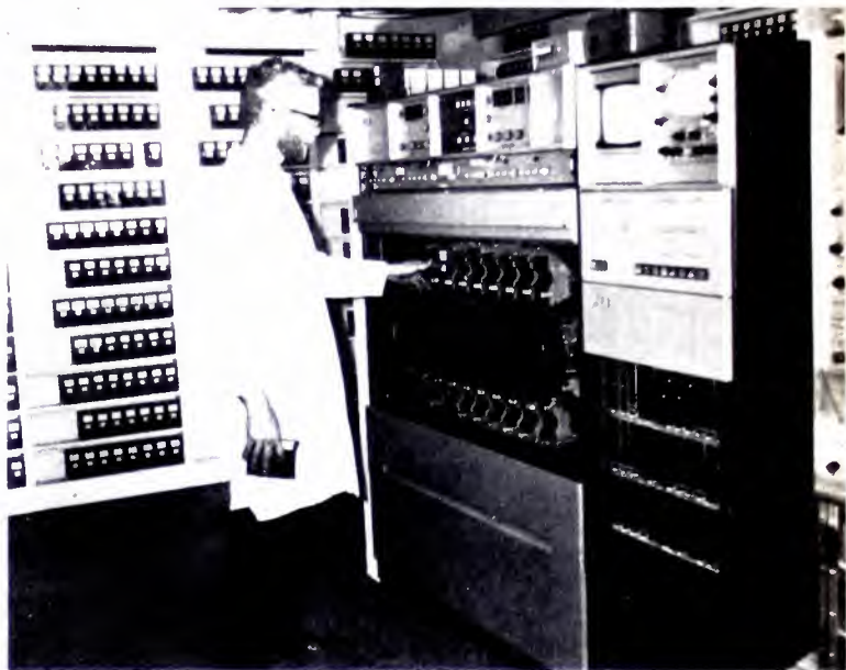
Inserting a "cart" into the TCR-100 for making a dub at KOB-TV.
