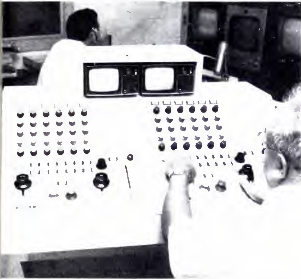
Control panel and console for two-camera remote control system at WHEN-TV, Syracuse, New York. The console is portable and movable between two Control Rooms. Each camera features six "shots" complete with manual hand controls.
