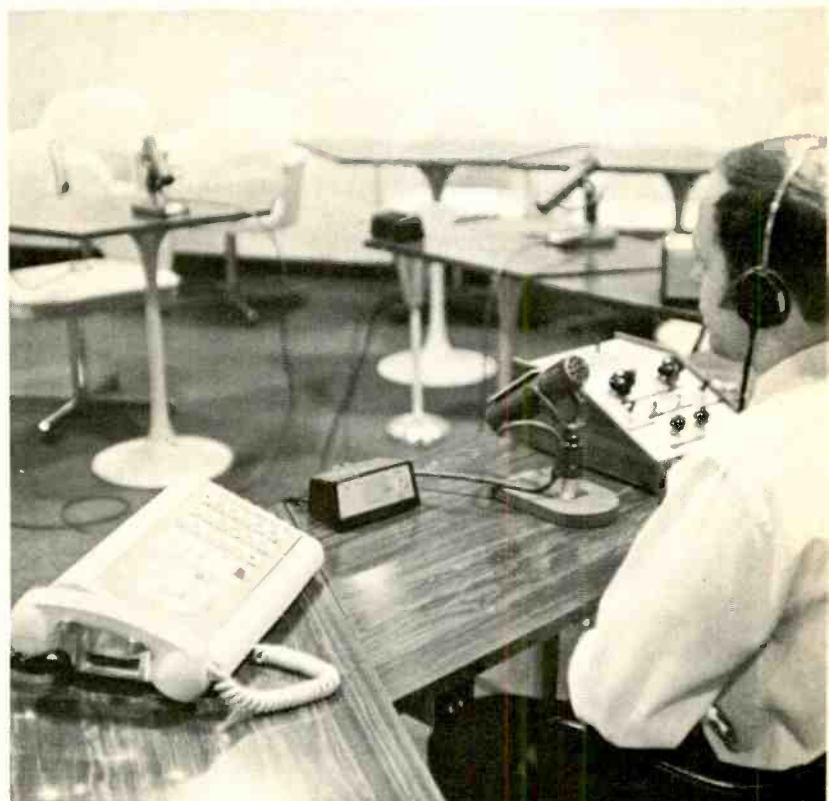
Fig. 1. View of call director, speaker/phone unit, mike, and announcer turret at WMCA.
