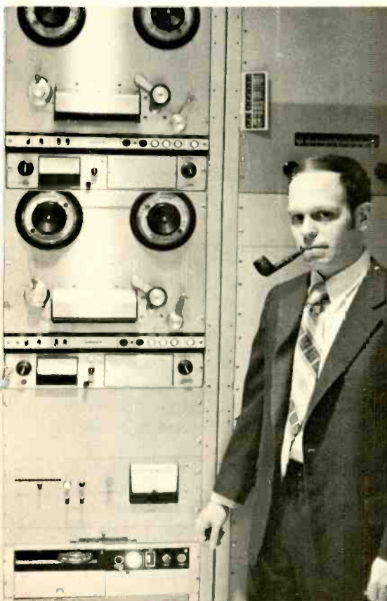
Fig. 4. Bob Kanner in front of delay transports. Seven second cart player is at bottom of rack.
