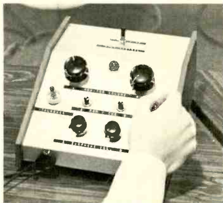
Fig. 2. Closeup of announcer turret showing on-off mike switch, top row; attention light (from producer) between monitor speaker volume controls A and B, second row; Talkback switch, Cue A button, Cue B button and cough switch (concealed), third row; Earphone volume controls A and B, bottom row.
