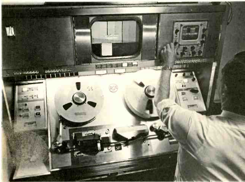
Equipment photos at NBC. Closeup of the TR-70 VTR and the complex master control room.
