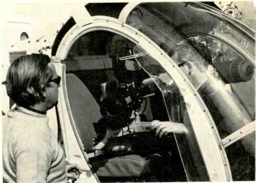
Special Tyler camera mounting fits Airflex-M 16-mm camera into helicopter. Ron Stewart (left) and KET cameramen go to great lengths sometimes for an unusual bit of footage.
