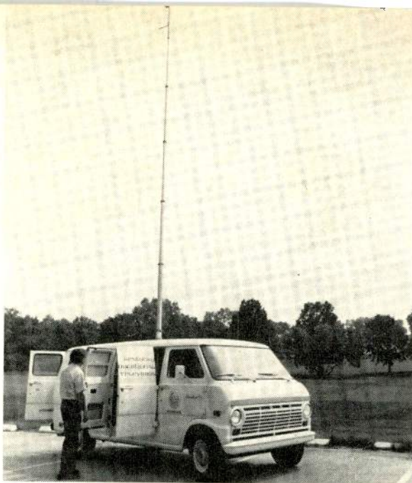
Field services truck surveys field strength with reference dipole on telescoping mast. Truck has own AC power to run test instruments inside. KET also surveys transmitter patterns with helicopter.
