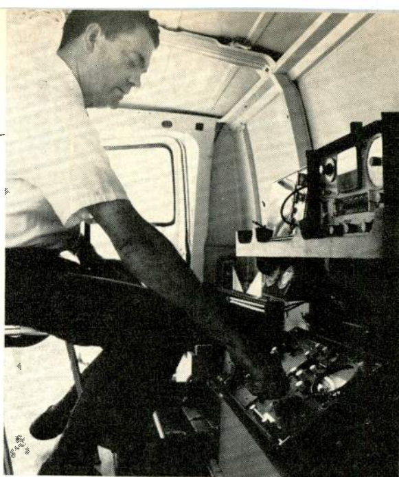
Engineer Paul Smith begins set of field tests with type-approved Empire meter. Jerrold model 727 backs up main instrument and serves when portable unit is needed.
