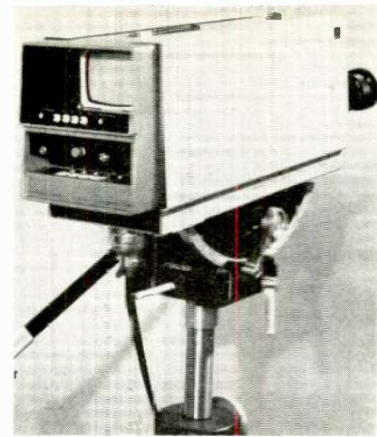
Low-cost color camera, IVC-100, has electronic viewfinder, sync gen, encoder, $14,000 price tag.
