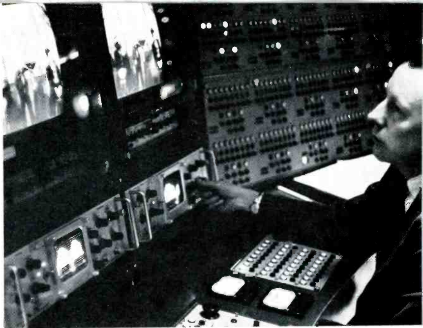
Test signals originate at NBC's New York master control, and are displayed on panel scopes.
