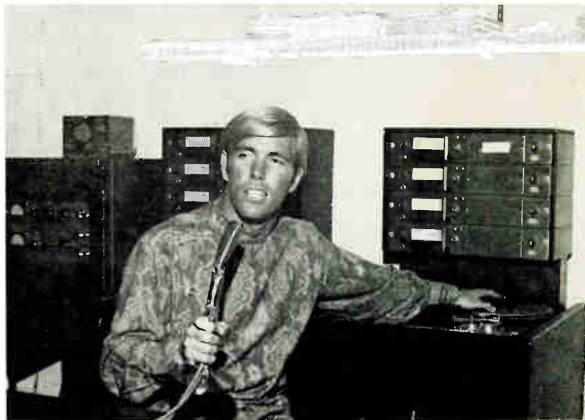
Well-tanned deejay pretapes his show using Ampex four-track recorder. Show will be aired from automation rack.
