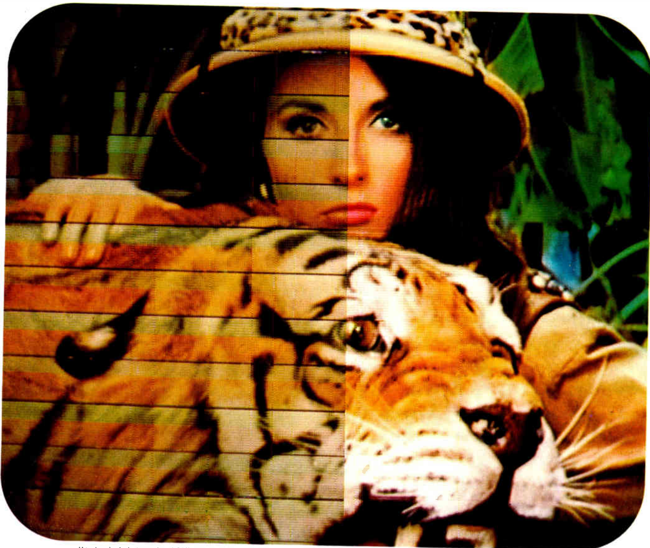
Unretouched photographs of 21" studio monitor. Photographic data: Rolleiflex C-3, CPS color negative film — ASA 100, 1/15 second at f/5.6
