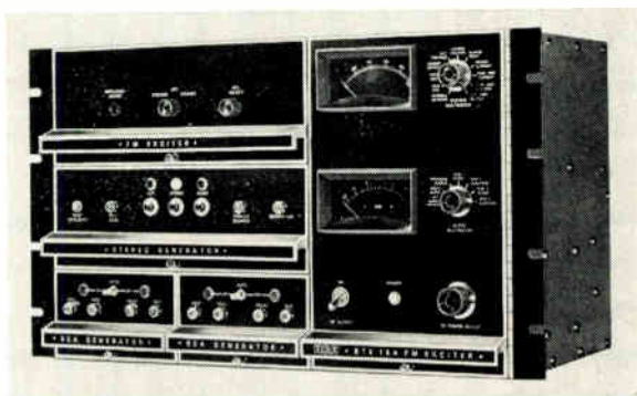
RCA's BTX-1B SCA multiplexer mounted in direct fm system offers deluxe features but is typical in its modular construction. The Marti SCG-67 (below) is directly rack mountable.
