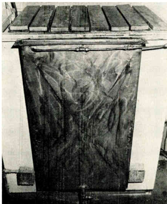
Water jacket holds seven deep tanks, uses coffee-pot heating elements to keep solutions at proper temperature.
