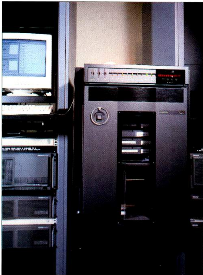
The Ampex DST 412 library storage system, fully integrated with the Tektronix Profile video server, runs under Louth Automation. The DST 412 automated cartridge library provides an optimum balance of system performance, cost of storage, and manageability.
