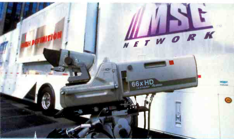
National Mobile Television's HD-1 is an all-digital, high-definition mobile truck. Here it is parked outside New York's Madison Square Garden with a Fujinon 66X lens shown in the foreground on a Sony HD camera. (Photo courtesy of Fujinon.)
