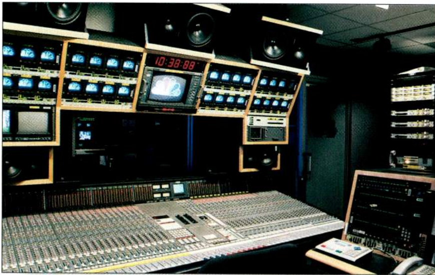
Most news broadcasts can be handled by a small console. This NBC news Washington audio control room shows how network demands require a more extensive setup. In this case, an SSL 8000 GB is integrated with a wide variety of support technology and multichannel mixes to handle any assignment. (Photo courtesy Communications Engineering Inc.)
