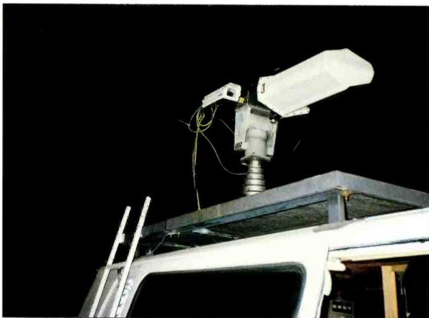
A 30-foot pneumatic mast with a pan/tilt head, Scala yagi antenna, rotator, compass and B&W camera was used at each measurement point. The camera image provided a picture of what the receive antenna "saw" as it looked toward the transmitter site.
