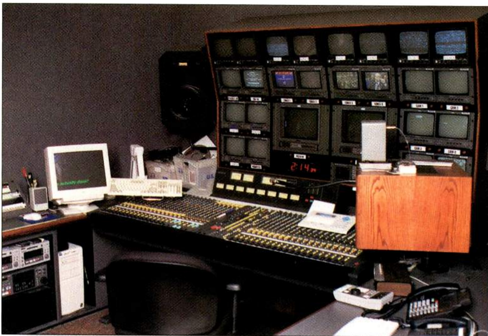
The main audio production room provides full AC-3 and 5.1 surround capability supported by a Sony MPX-700 console.
