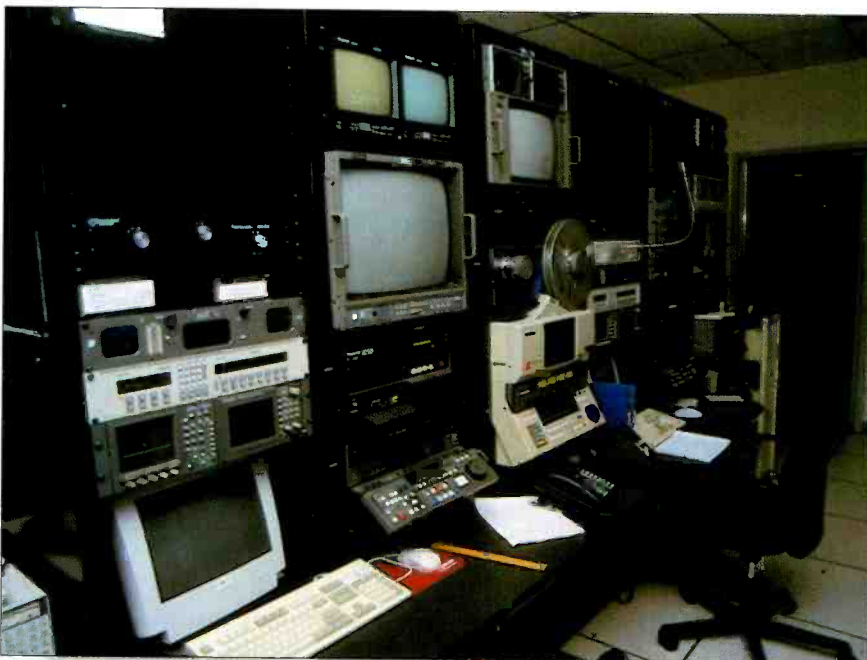
Lifetime's ingest stations include ready access to a variety of tape formats, making it quick and easy for operators to transfer tapes to files.
