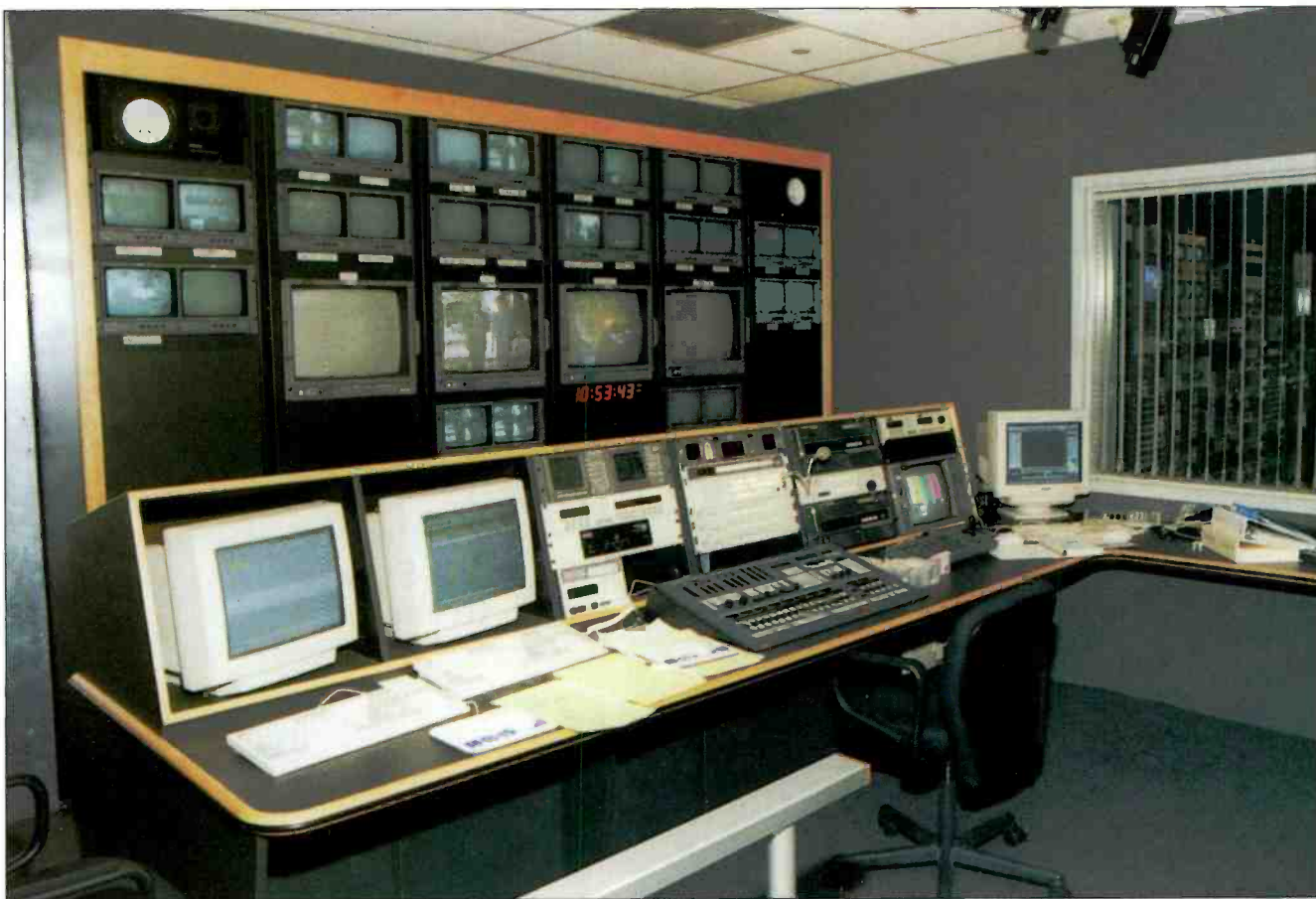
One claimed benefit of automation is that more (typically channels) can be controlled with less (typically people). Note the simple, straightforward layout of this control room at Lifetime Television. Such a design can allow one person to handle ingest, archiving and on-air operations if needed. Typically these tasks are divided between several studios, which provide other types of efficiencies.
