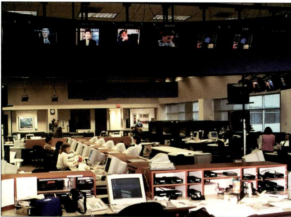
The WSB newsroom uses Avid News with individual editing stations for all working journalists. The system is tied to a Sony BZN-5000 server system using dual servers, a news server and an on-air server. The 12 linear editing bays will soon be updated with clip edit capability where last-minute edits automatically update to the on-air server. The room provides two on-air broadcast locations, so news updates can be handled directly from the working newsroom.
