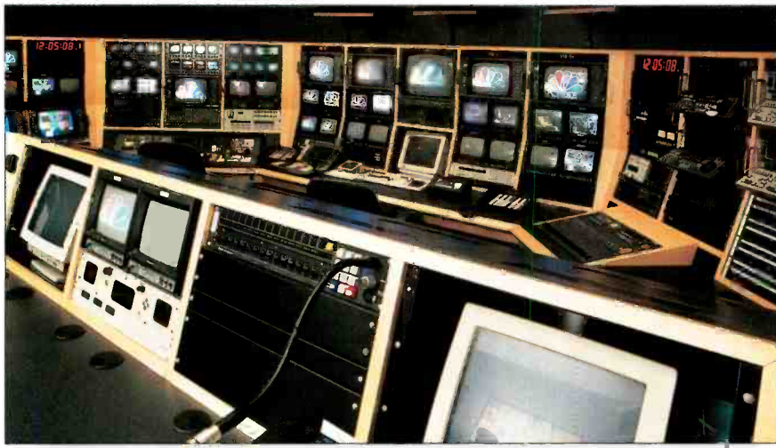
Today's graphic suites, like this one at NBC News Washington, often operate like small production islands. However, best efficiencies come from interconnecting them to the rest of the facility with 601 interfaces so all areas can take advantage of the staff's creativity. A key advantage in building with 601 now, is the longer life and future options it brings to both user and facility. (Photo courtesy Communications Engineering Inc.)
