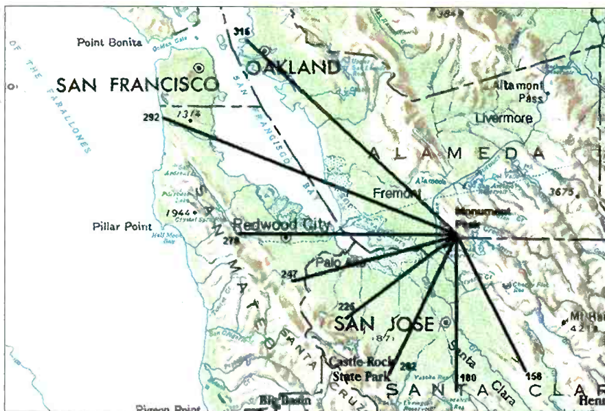
Map shows the eight radials tested. All denote the compass heading from Monument Peak. The 76 test sites on these radials ranged from 2 to 37 miles from the transmitter site. Measurements along the radials stopped when that radial reached water or a mountain ridge.
