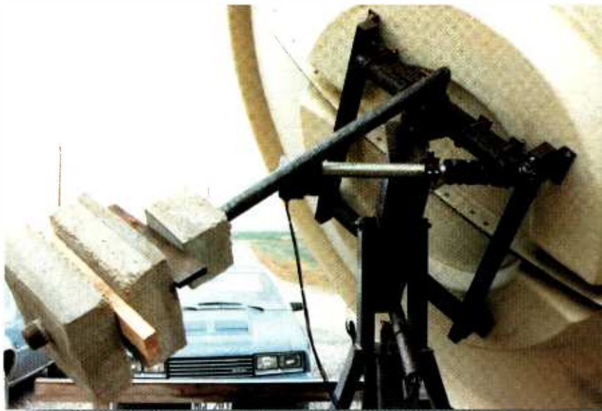
The counterweights were mounted on a five-foot lever arm and provided enough weight to offset the weight of the dish.
