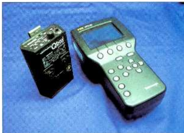
The Tektronix WFM 90 is a hand-held video monitor that can show audio and video waveforms, vector displays and picture-in-picture.
