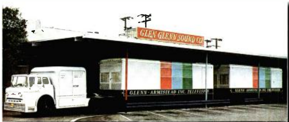
Tractor and two trailers that comprise the Glenn-Armistead color TV production system. One unit contains control, switching and effects equipment; the other contains a film system and two color TV tape recorders.
