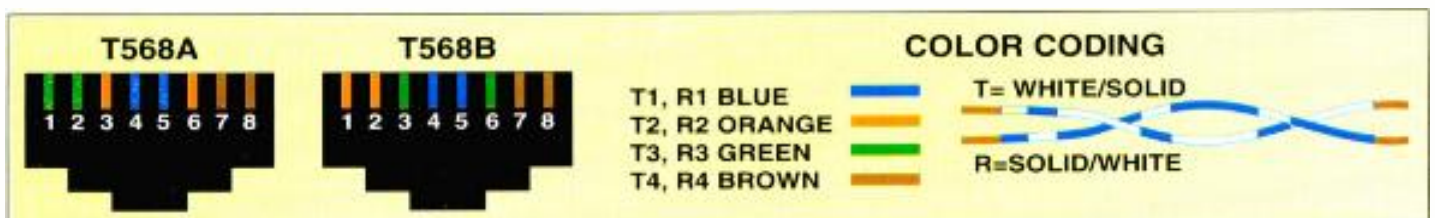
When wiring 10 Base-T Ethernet connections, only two pairs of conductors are needed. One pair connects pins 1 & 2, the other pair is for pins 3 & 6. However, cabling for network applications typically has four pairs. Standard connections are shown, the T568A configuration is preferred, and directly compatible with two-pair voice and token-ring systems using six-position connectors. The T568B method is optional and directly compatible with AT&T phone systems.
