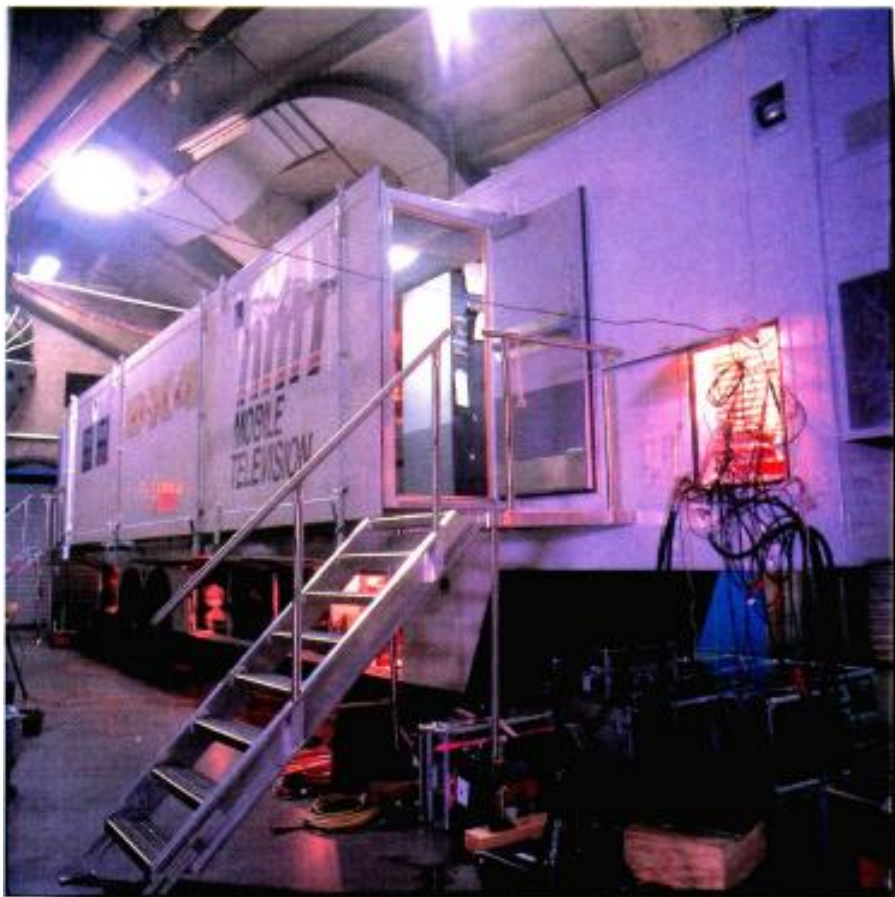
Flexibility is the key to success for mobile production units. Well-designed I/O panels, along with the ability to quickly add to or change the equipment configuration increase a vehicle's flexibility.
