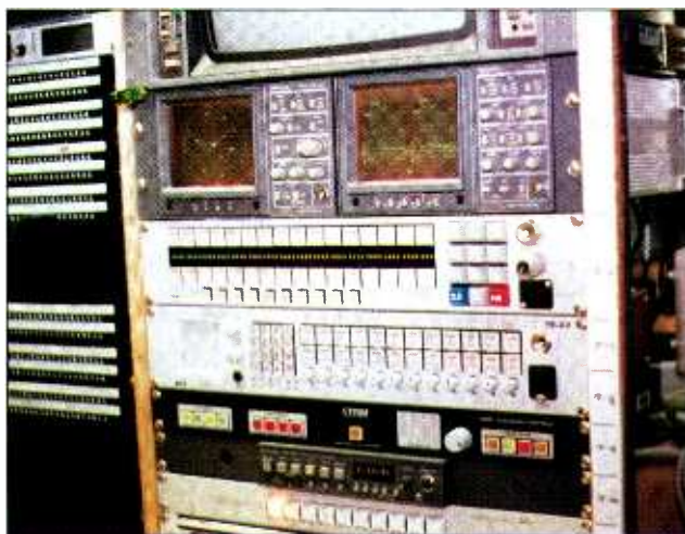
The truck's transmission/QC rack provides centralized and distributed intercom architectures. Shown here are the RTS/Telex 803 TW master station and KP98-7 ADAM key panel.
