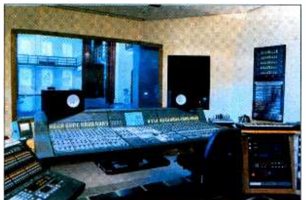
At La Chapelle studios in Belgium, a Euphonix CS2000 provides digital control of analog audio signals.
