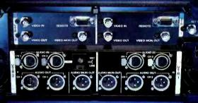
•Mic and line level inputs •Video in/out and monitor out •RS-422 control ports • Line audio and monitor outputs
