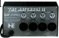
Get Matchbox II to convert "consumer" (RCA and mini-jack) audio inputs and outputs to "600 ohm" balanced lines at +4dbm professional levels. Eliminate the hum, buzz, and distortion caused by mismatched levels and impedances! Gold plated connectors and direct-coupled, active circuitry yield superb audio performance. Over 20,000 units in use worldwide!
