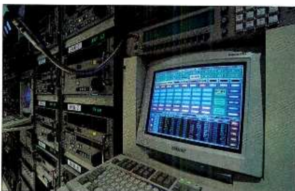
A close-up of one of the touchscreen workstations, note the EWT displays in the background.
