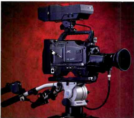
The JVKY-27, set up in a studio configuration. Many facilities are opting to use EFP-style cameras for studio use.
