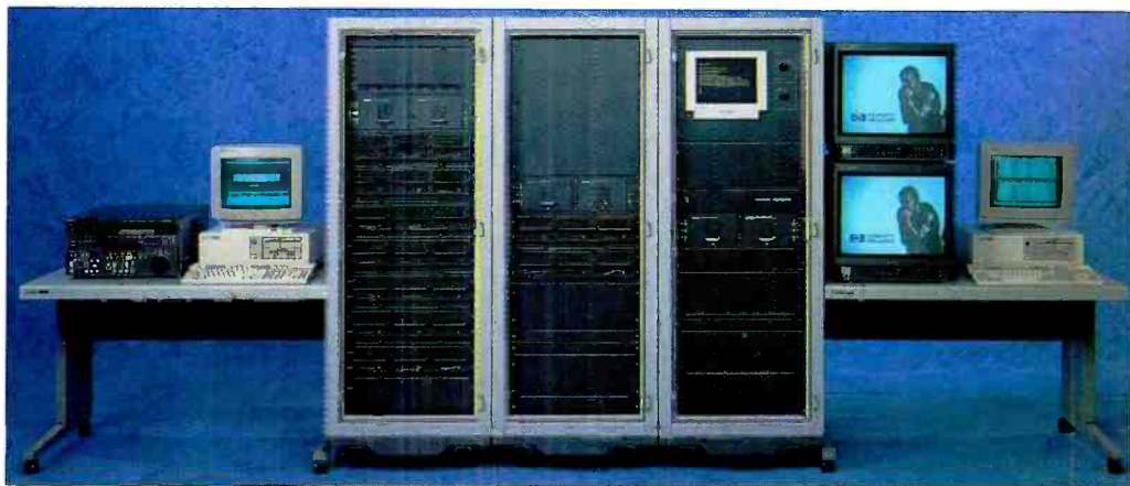
Hewlett-Packard Broadcast Video Server capable of storing six hours with up to 51 hours available as an option.
