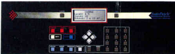
4YDM control panel
