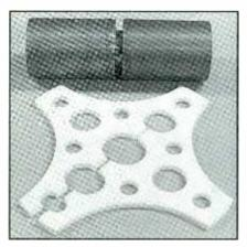
Figure 1. Old-style insulator and undercut.
