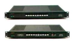
RS-103 Series Routing Switchers. Our versatile 10x1 routing switchers come with 40MHz bandwidth, remote and RS-422 control and may be configured for component and matrix switching. The RS-103A also gives you three channel audio-follow-video.
