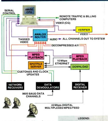
Figure 1. Digital satellite delivery of commercials can tie even the most remote cable systems together as an interconnect, or transport national and promotional spots for near immediate turnaround.
