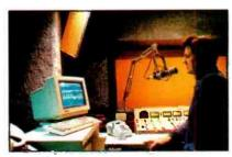
A PC-based radio automation system in use. (Courtesy of WIBW-FM, Topeka, KS.)
