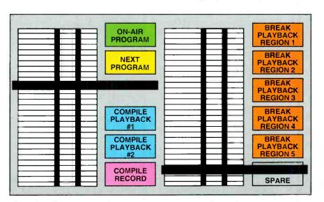
Figure 3. VTR allocation and layout of a cart machine system for multiregional spot insertion.
