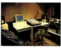
A radio production studio using a virtual multitrack digital production system in an analoginterfaced application.
