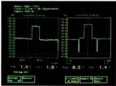
Figure 5. Detail measurements show the amount of overshoot or rounding of fast transitions between black to white.
