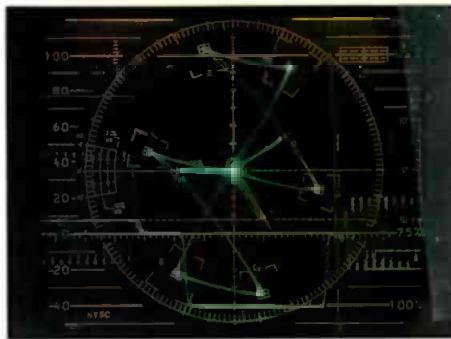
The standard vector display shows chrominance amplitude and phase angles of SMPTE color bars.
