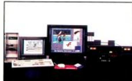
This desktop video package consists of an EISA-bus PC and a set of five plug-in cards. The proprietary software for hardware resource management runs under the Microsoft Windows 3.1 operating system.
