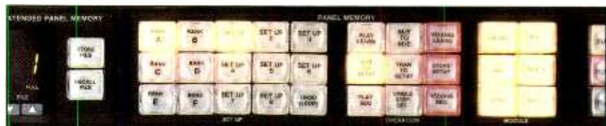
SuperSTAR panel memory allows quick recall of preset effects. (Courtesy of Ampex.)
