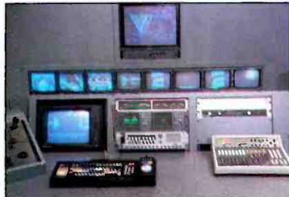
The operator's position at Vidcom Post, Burbank, CA. Editor control is to the left, and the audio mixer is to the right. Intercom is at the center.
