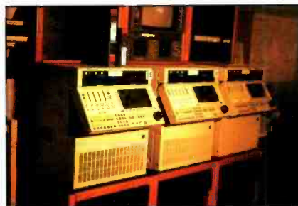
Digital composite tape machines were originally designed to replace analog composite VTRs. Innovative facilities use digital to increase the quality of video production.
