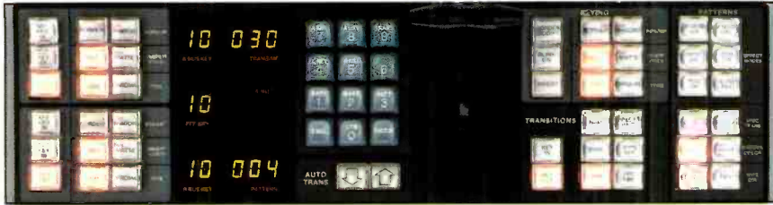
Each M/E has three full-capability keys: one for each bus and an effects keyer. (Courtesy of Ampex.)
