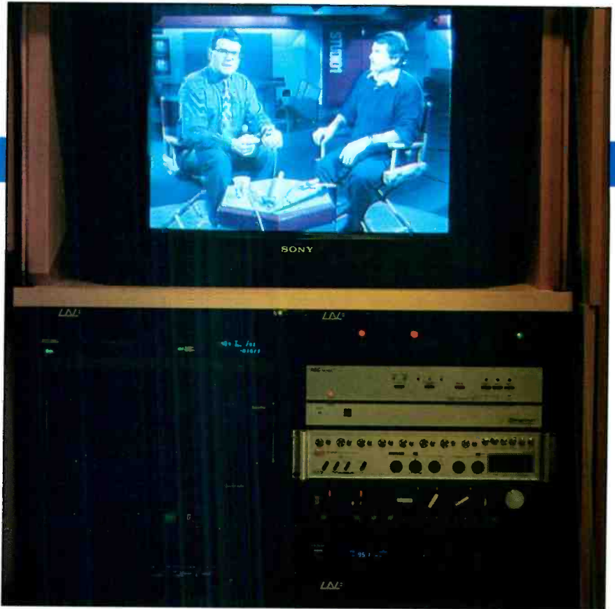
The user-operated equipment rack includes surround decoder, video laser disc players, S-VHS recorder, audio equipment and a professional video scan converter. (Courtesy of Don Dutkowski.)
