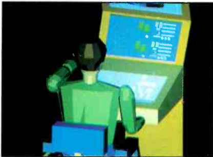
Figure 13. A console with a high desk forces the user to spread arms out, which forces wrist positions to angle toward the little finger (ulnar deviation).
