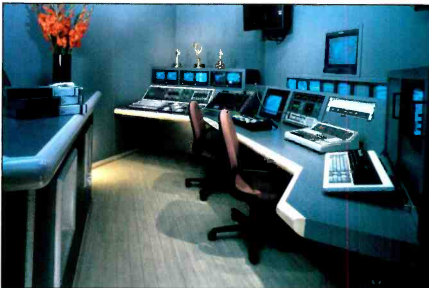
A new composite digital edit suite at Vidcom Post, Burbank, CA. The switcher is to the rear, on the left as you enter the room. The digital effects system is to its right. The edit controller is the black keyboard in the center. The audio console and character generator keyboard are in the foreground.
