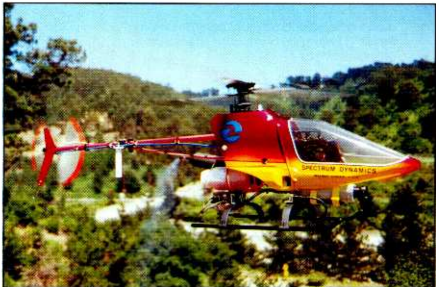
Side view of RPV ENG helicopter shows the camera beneath the cabin, the 2GHz transmitter located below the fuel tank and the omnidirectional ENG antenna on the boom near the tail rotor.
