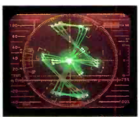
Triple Vector Overlay— SMPTE Bars on A, B and C inputs delayed by 6° and 12° to demonstrate phase error
