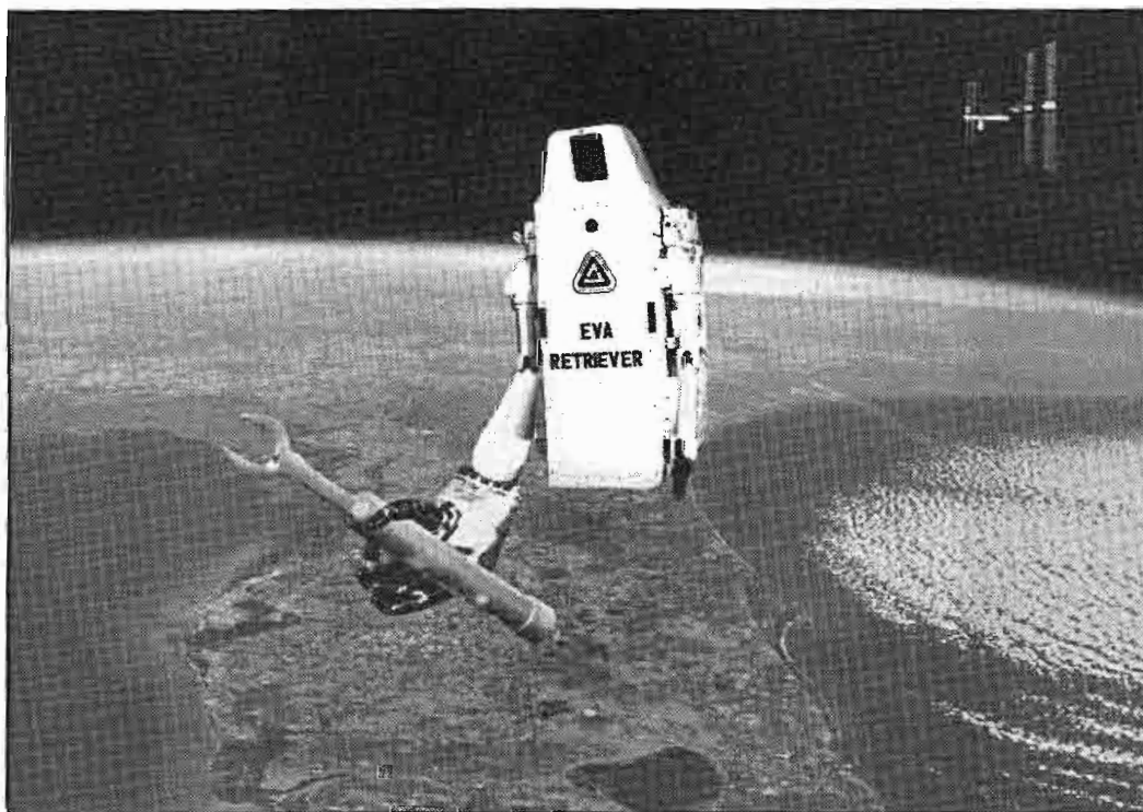
An artist's depiction of EVA retriever with "smart hands." The robot will fetch tools and components "dropped" by astronauts.
