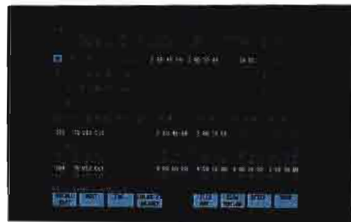
A 2-channel, 3-band equalizer is available on the optional internal audio switcher. Once displayed on the monitor, each equalizer channel can be adjusted individually with the shuttle/jog knob.
