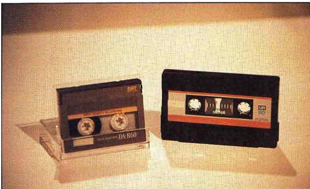
The smaller cassette size is deceiving. Each R-DAT cassette is capable of providing two hours of stereo recording.
