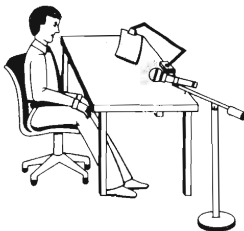
Figure 1. Many of the acoustics problems broadcasters face begin with copy stands, counters and windows. As the announcer's voice reflects from these surfaces, the timbre is changed, making it sound unnatural.
