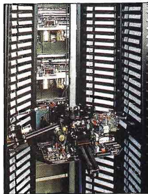
The library tower and robot arm manipulator open for inspection. The octagonal design and 4-arm manipulator make short work of loading and unloading carts.
