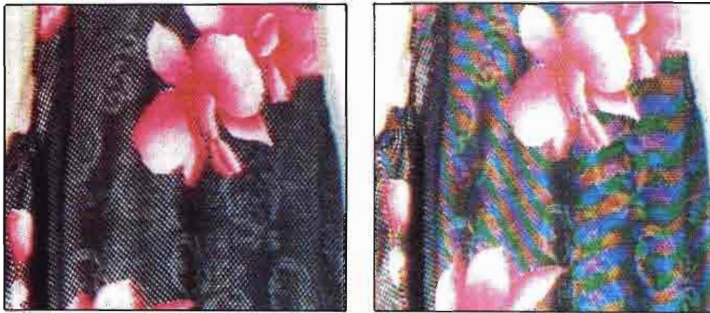
Figure 2. Cross-color artifacts introduce spurious colors into detailed scenes. (Photo courtesy of High Resolution Sciences.)
